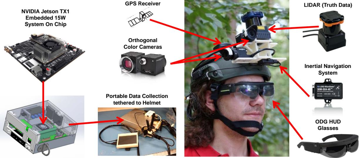
Figure 9. Various components of the helmet mapping system. The Jetson board is tethered to the helmet and carried by a shoulder strap.
