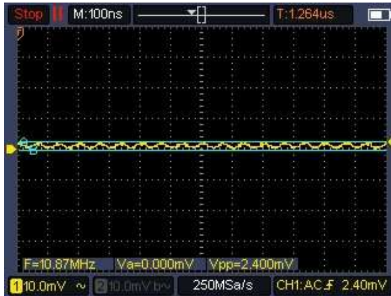
Figure 33. Attenuated signal with low-pass filtering.
