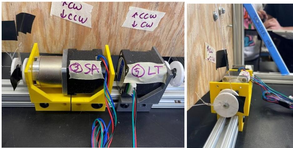
*Figure 62: Serratus anterior motor mount (yellow) and lower trapezius (gray) shown with motors and fishing line spools installed*
