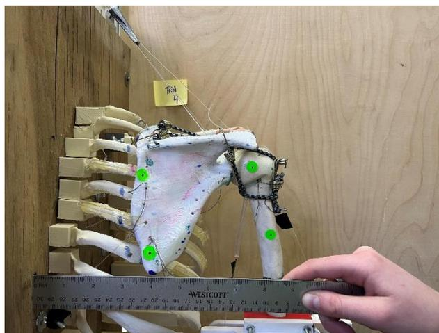
*Figure 68: Example of photo tracking dots used in testing*
