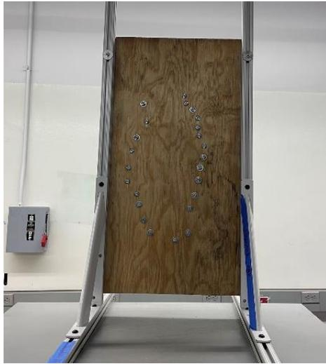
*Figure 57: Back of the assembly showing bolts from the rib connections, t-slot beam supports, and plywood*
