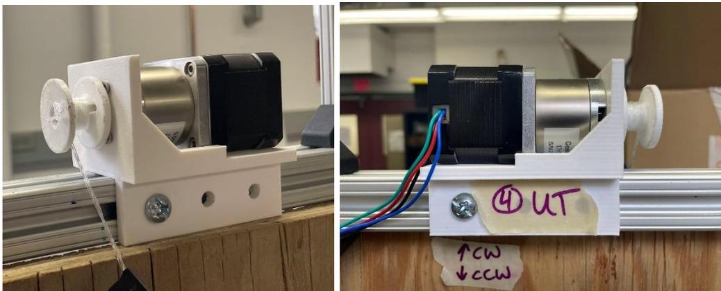
*Figure 63: Upper trapezius motor and mount shown from the front side of the board (left) and the back side of the board (right)*
