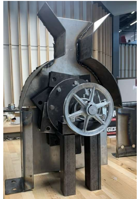
Figure 3, the grinder that our colleagues built to process PCBs.
