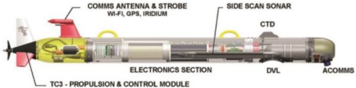
Figure 5: Design of HarborScan [10]
