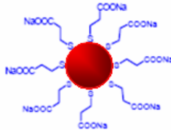
Figure 4: Diagram of quantum dot with coating that allows water solubility
