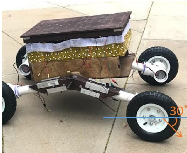
Figure 35: Infrared Range Finder Placement Angle
