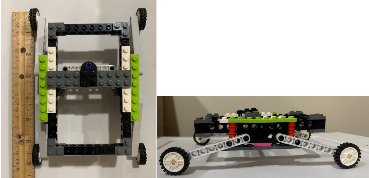
Figure 14: Rocker Scale Model Top and Side Views
