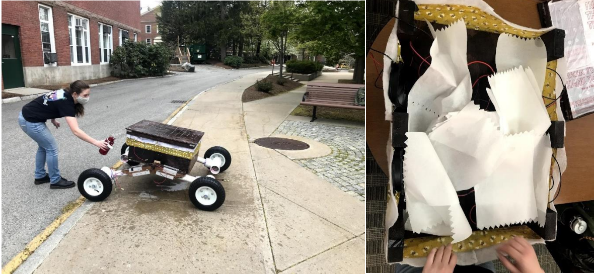
Figure 34: Water Ingress Testing and Results
