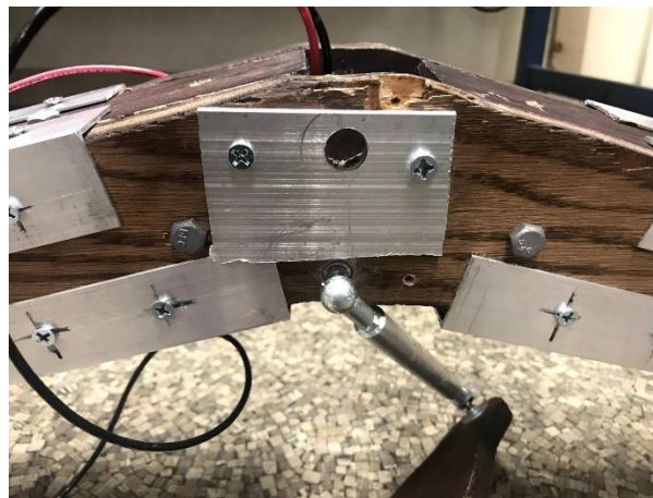
Figure 40: Reinforcing Aluminum Plates
