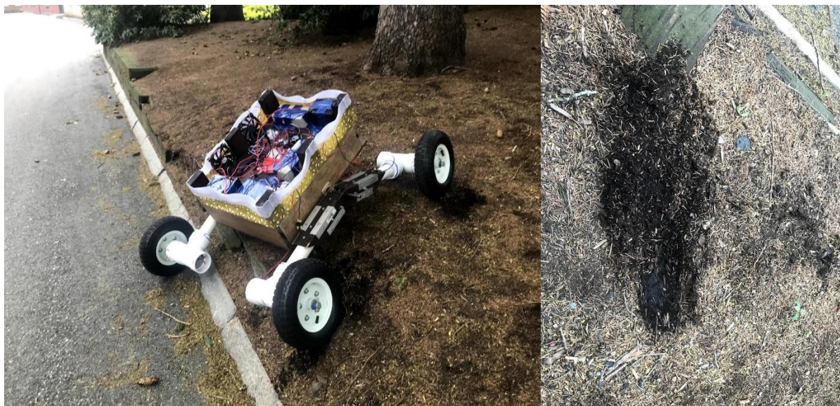
Figure 38: Drivetrain Testing in Loose Ground
