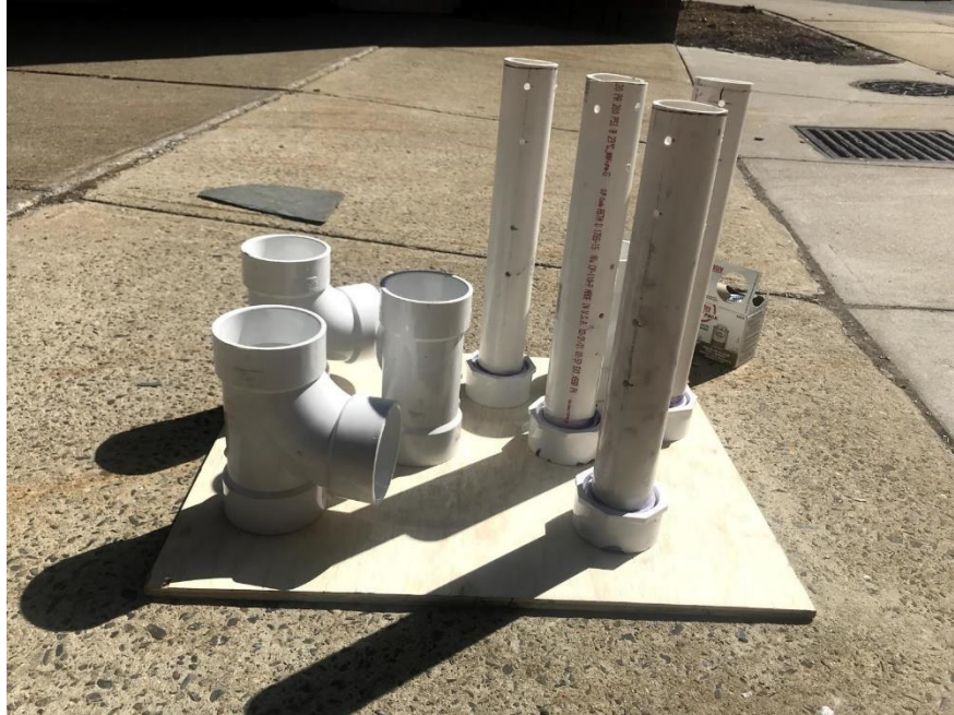
Figure 15: PVC Solvent Welding Setup
