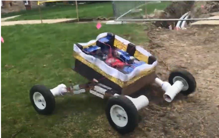
Figure 37: Drivetrain Testing in a Ditch
