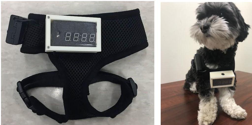
Figure 6.1. Final cough counting device mounted on a small dog harness, and being worn by a canine meeting the physical criteria of our targeted patient.
