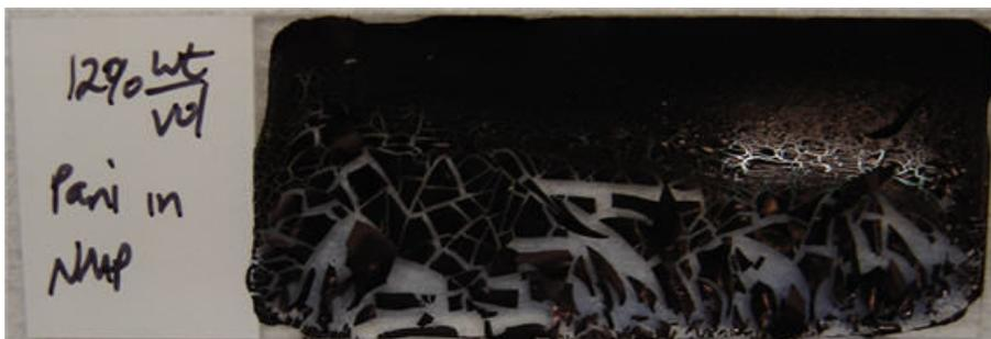
Figure 17: 12% wt/vol PANI Film That is Highly Cracked
