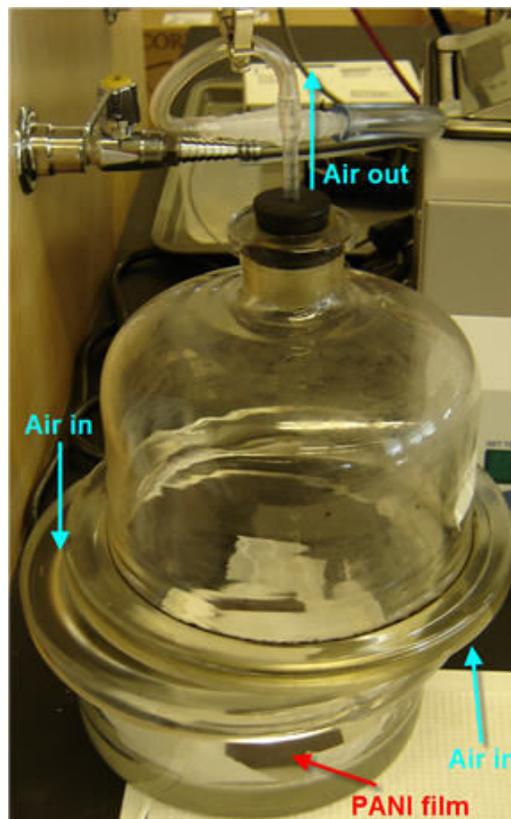
**Figure 10: Set Up for Manufacturing PANI Films**
