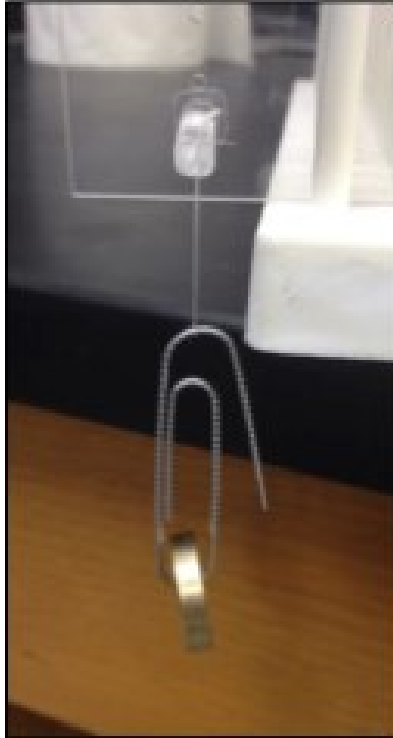
Figure 5.4: Picture Taken From PDMS Anchor Point Loading Testing
