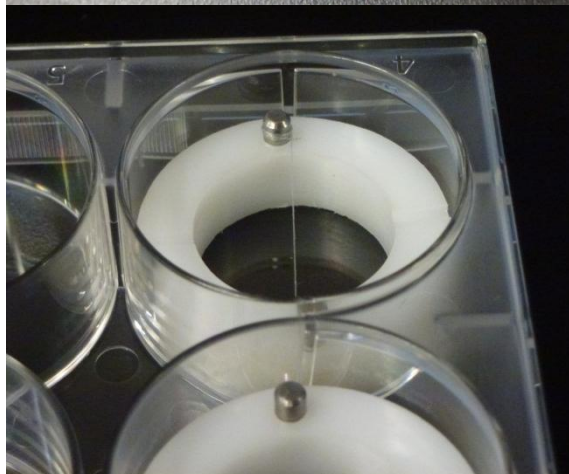
Figure 31: Delrin ring assembly inside wells of a six well plate. The top image shows 2 assemblies placed in wells of a six well plate, one with the thread bundle mounted (top well), and one without the thread bundle. The image to the left shows an angled view of the assembly inside the top well for better depth perception.
