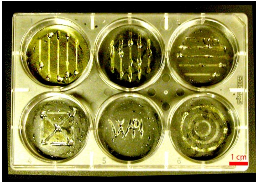
Figure 6: Programmed patterns printed by the cell printer inside wells of a 6-well plate using 1% Sodium Alginate. Top row: left to right: 2 wells with vertical parallel lines, 3 rd well with horizontal parallel lines. Bottom row: left to right: square with diagonals, the letters WPI, 3 concentric circles.
