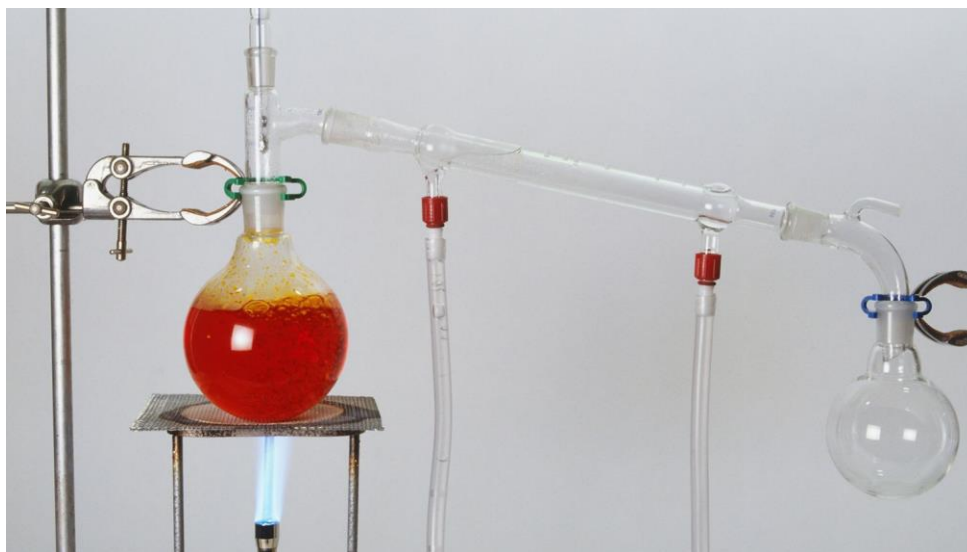
Figure 2.6.1A: Photo of an example distillation (Kindersley, 2019). Here, the orange solution is being evaporated, the gases from which are traveling through the long tube on the right where they condense and collect in the other flask.
