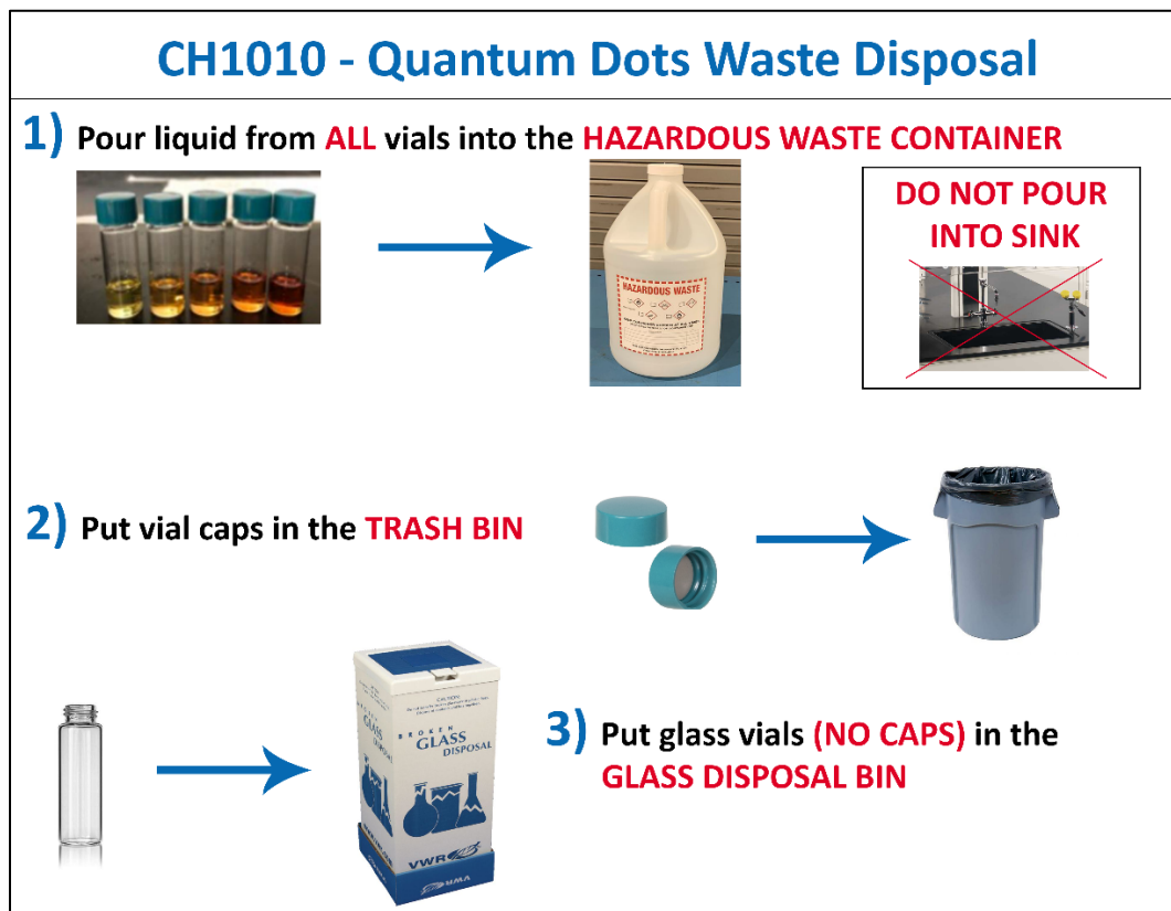
Figure 5.3.3A. Example of a specific waste disposal poster that applies to one of the experiments in CH1010 .
