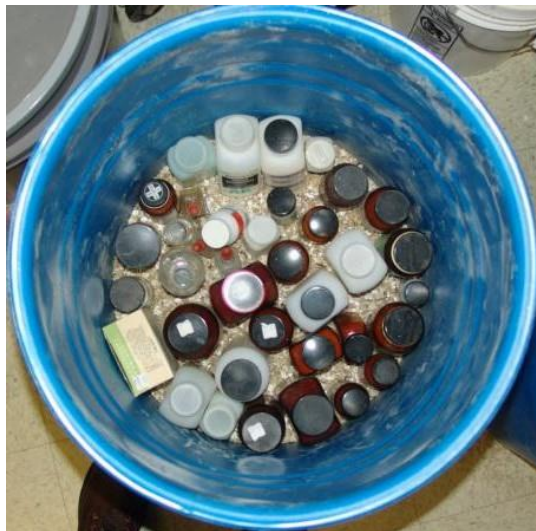
Figure 2.3.3A: Photo of a lab pack ( Mountain States Environmental Services , n.d.). In this case, the pack is a steel drum containing various chemical bottles surrounded by an absorbent material.
