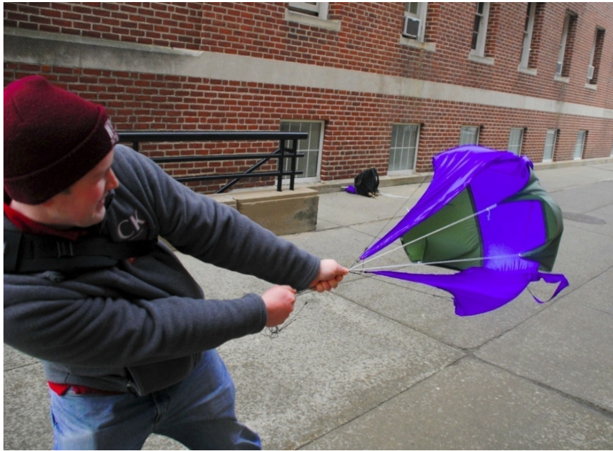
Figure 39: Sailwing/cross parachute testing in an outdoor, semi-channeled flow
