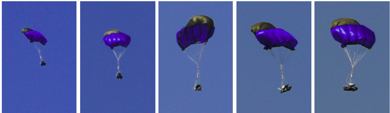
Figure 44: A series of images showing the parafoil as it descends in pre-transformation mode with a portion of post-transformation fabric partially deployed
