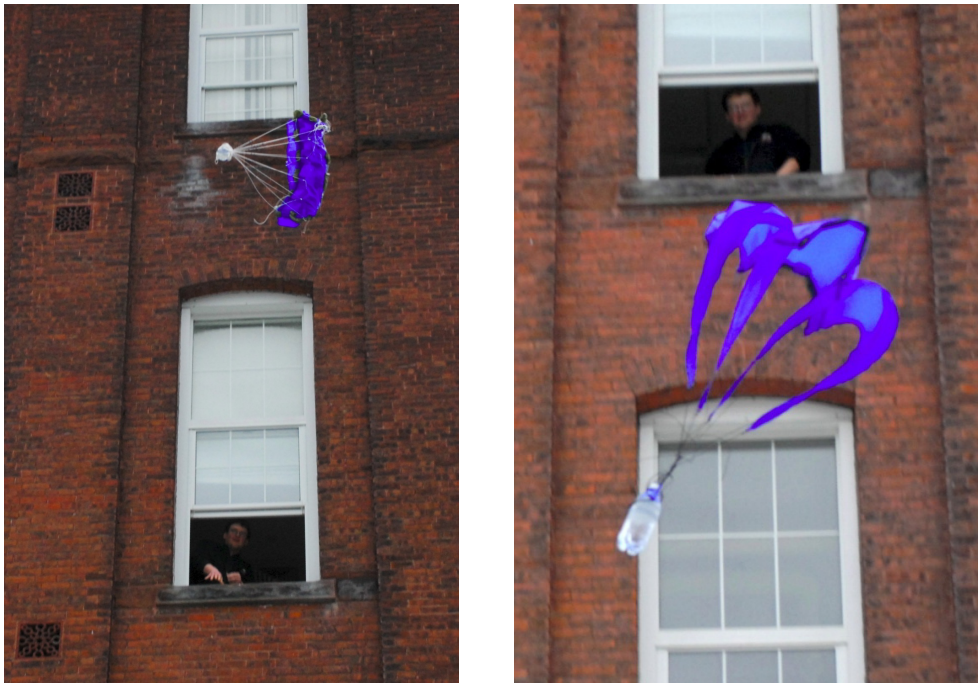
Figure 34: Drop testing the parafoil (left) and the sailwing (right) from Salisbury Labs
