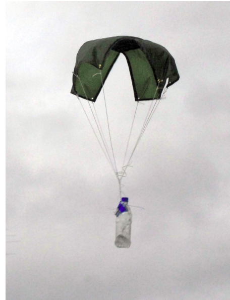
Figure 18: Prototype cross parachute constructed for wind tunnel testing
