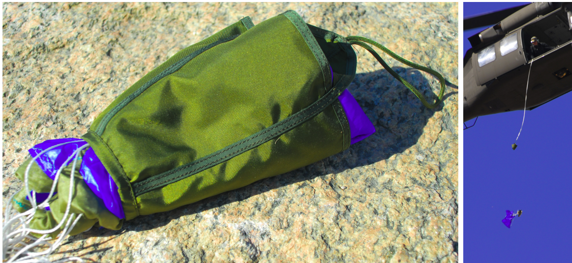
Figure 41: The parafoil packed into its deployment bag (left) and the sailing immediately after deployment from its bag at the end of the static line (right)
