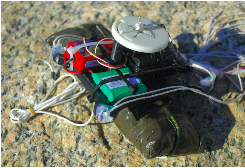
Figure 40: The payload package on the parafoil (identical to the sailwing's). Sandbag is olive green, receiver is red, battery is bright green, and servo-mechanism is black and white.
