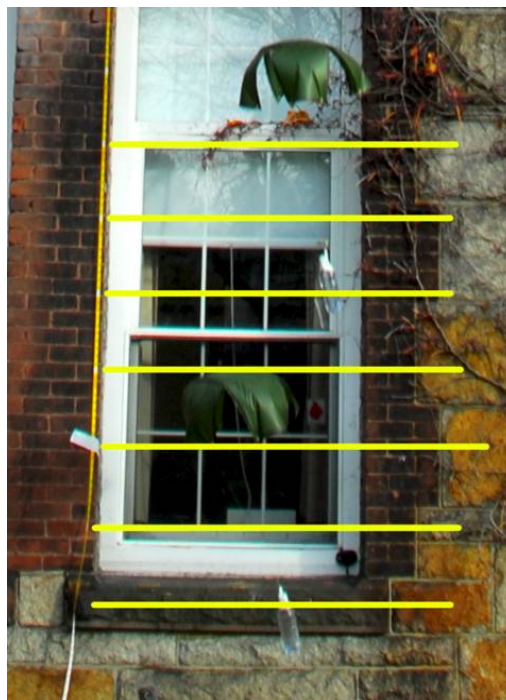
Figure 30: Drop test distance estimation, with frame overlap and enhancement done using Adobe Photoshop
