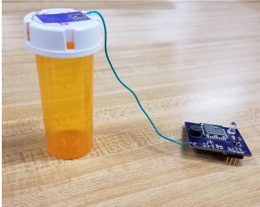
Figure 4.13: Finished prototype with PCB hardware and medication bottle.
