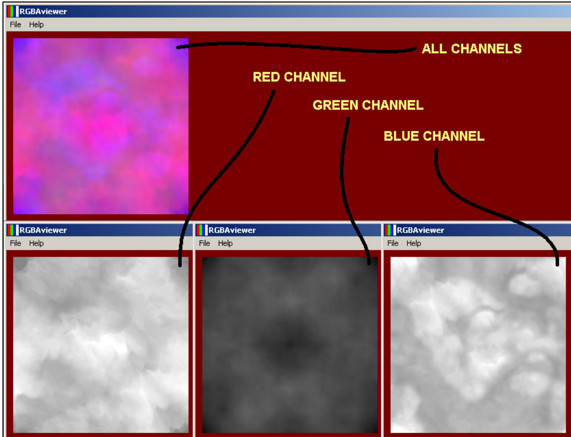
Figure 20: The different color components of the one texture used for the sky effect
