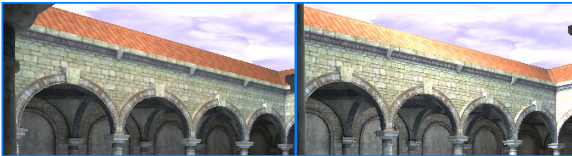
Figure 18: Screenshots with diffuse lighting only (left) and with specular lighting & normal mapping (right)
