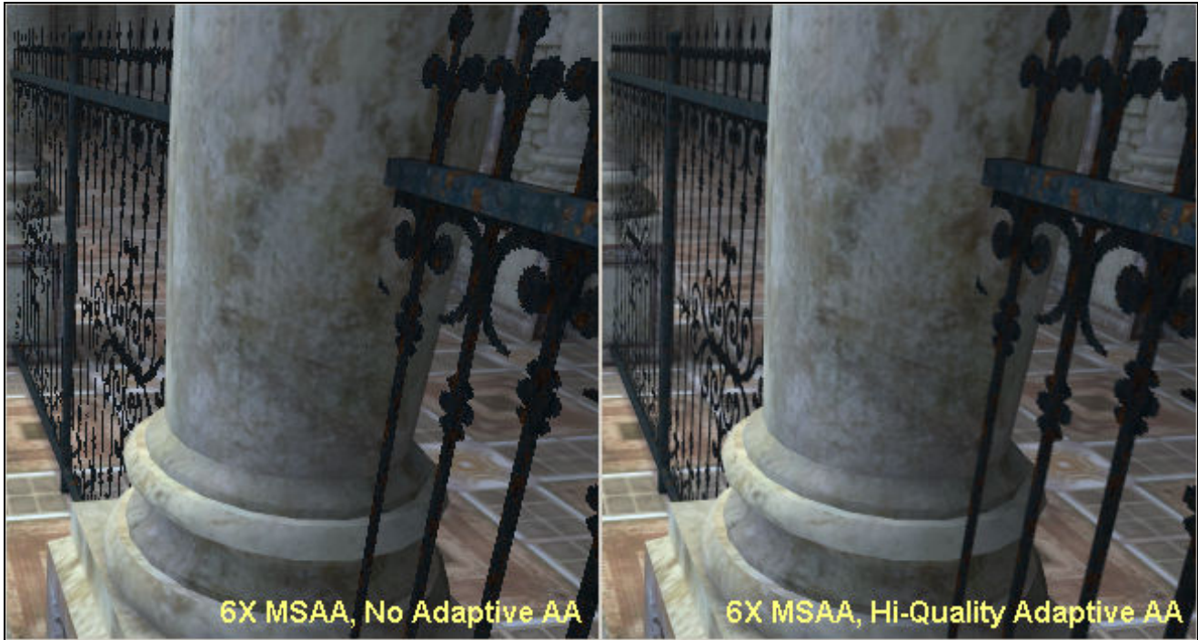
Figure 17: Fence with no adaptive AA (left) versus high quality adaptive AA (right)
