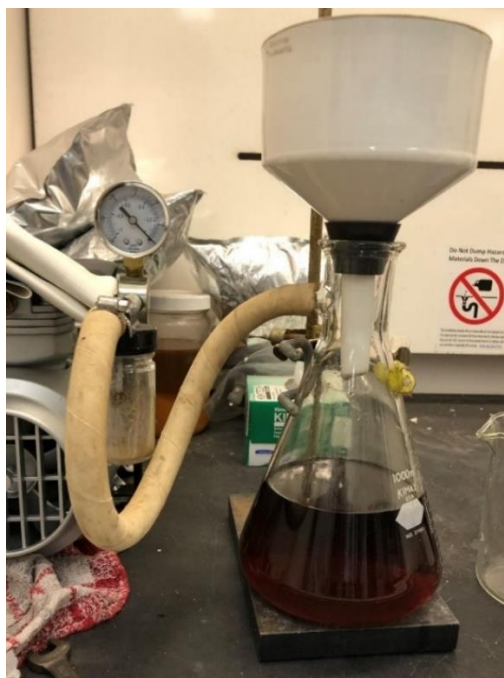
Figure 2. Vacuum filtration setup. The vacuum was connected to the 1000 mL filtering flask with tubing. A funnel was connected to the mouth of the flask, and filter paper (not visible) was placed in the funnel. The brown-colored liquid in the flask is the filtered DI water, ethanol, and soluble organic materials.
