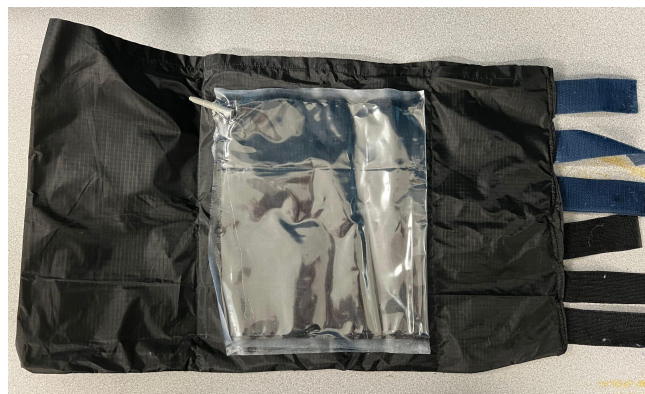
Fig. 4.3.3b. Cuff design highlighting bladder that inserts into the sleeve.
