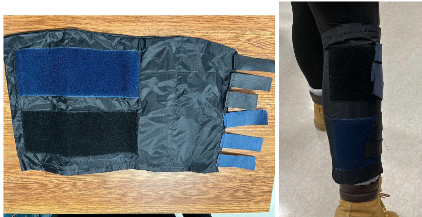
Fig. 4.3.3a. Cuff design highlighting overlap of Velcro strap mechanism for tapered muscles.
