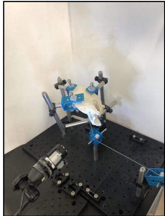
Figure 76: Clamp Assembly Static Testing
