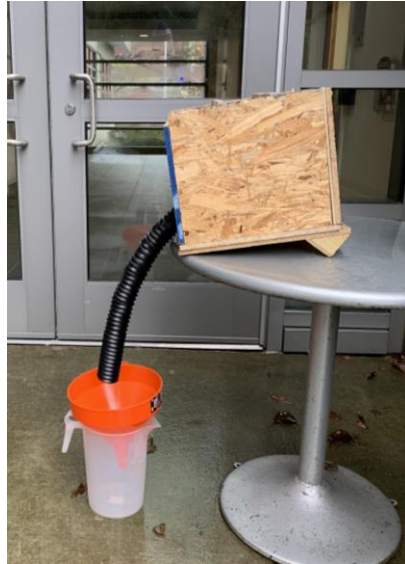
Figure 25: Drainage Test Setup with Tester Box
