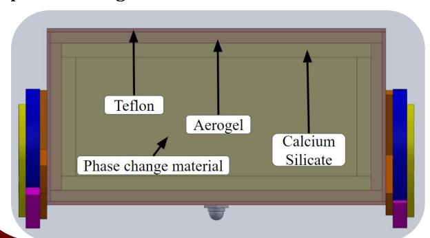
Requirement Metric: Maintain an interior temperature of under 60 °C:
