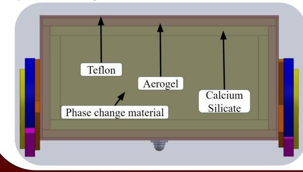
Requirement Metric: Maintain an interior temperature of under 60 °C:
