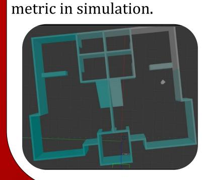
As a system test, the robot navigated through a virtual "fireground", created in Gazebo, for 15 minutes. The fire was modelled by the color on the walls, where the simulated temperature sensor would extract a color code to determine the temperature. The robotic model used included the following simulated components: camera, IR thermal arrays, radar, and battery.
