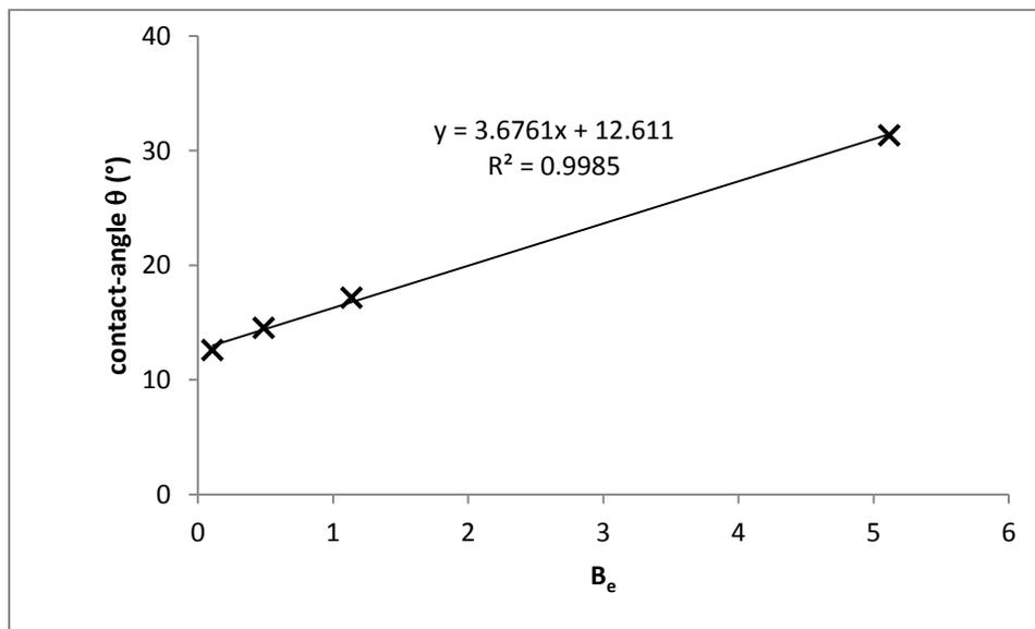
**Figure 3:** Contact-angles of PMMA-acetone solutions at all  $B_e$
