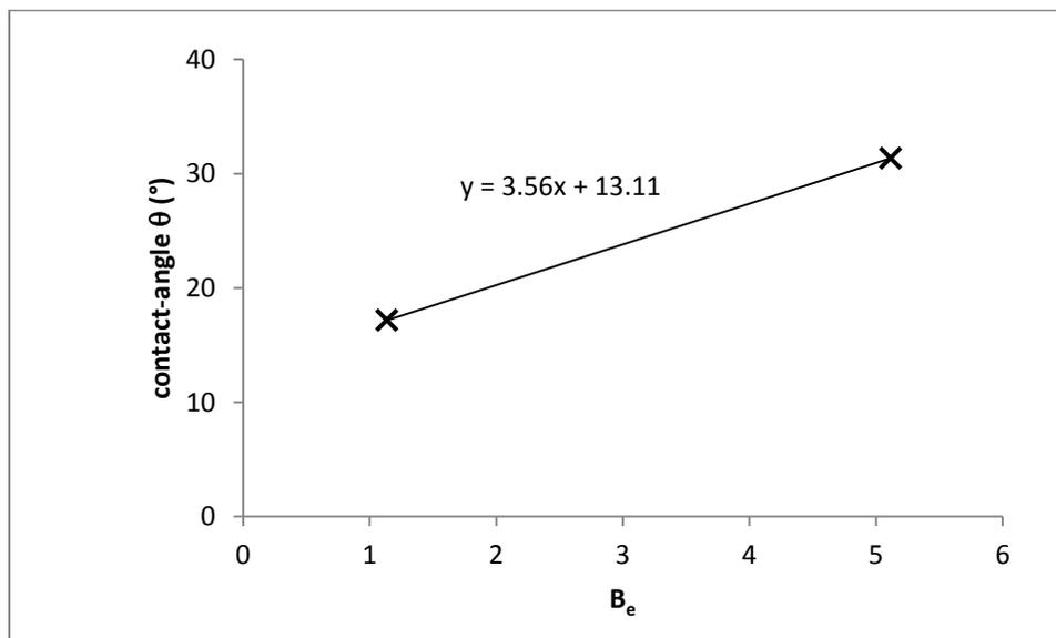
**Figure 5:** Contact-angles of PMMA-acetone solutions at  $B_e > 1$
