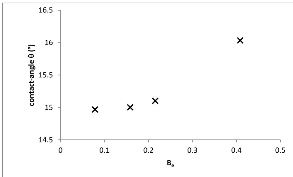
**Figure 7:** Contact-angles of PS-THF solutions at  $B_e < 1$
