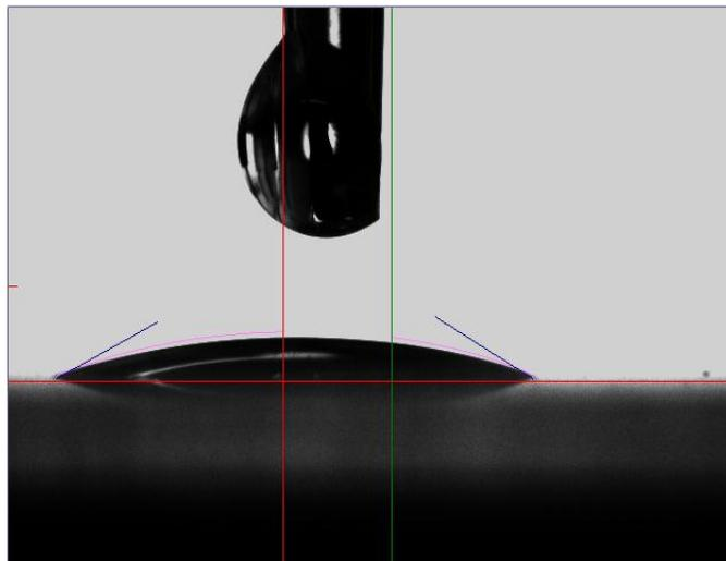
**Figure 2:** A droplet of 2% PMMA  $M_w=350,000$  on AAO template
