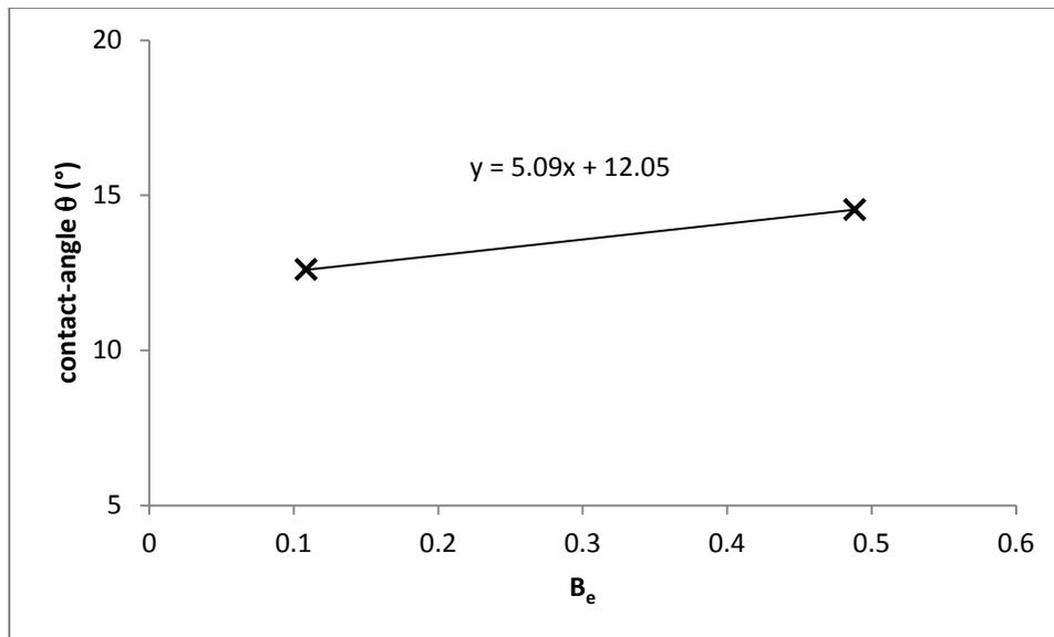
**Figure 4:** Contact-angles of PMMA-acetone solutions at  $B_e < 1$
