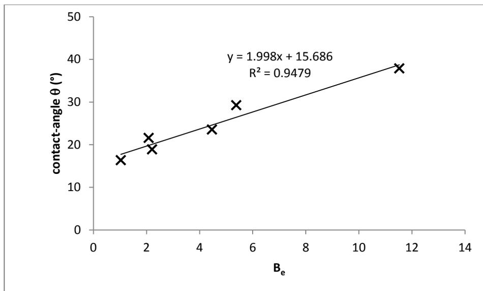
**Figure 8:** Contact-angles of PS-THF solutions at  $B_e > 1$
