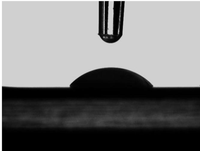
**Figure 1:** A droplet of 5% PMMA  $M_w=996,000$  on AAO template
