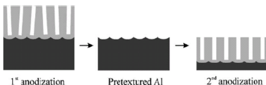
Figure 2.1 Schematic diagram of the two-step anodization process.
