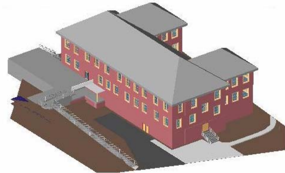
Figure 13: The 3 dimensional parametric building model for Kaven Hall, WPI as created using Revit
