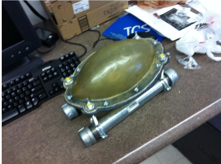
Figure 16: Prototype Fiber Glass Hull
