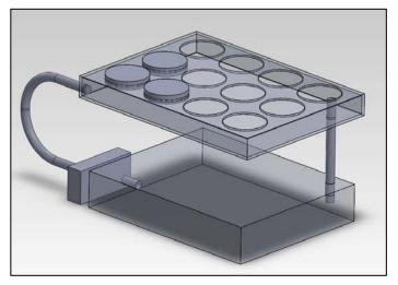
FIGURE 9: CAD DESIGN OF CONTINUOUS MEDIUM FLOW DESIGN
