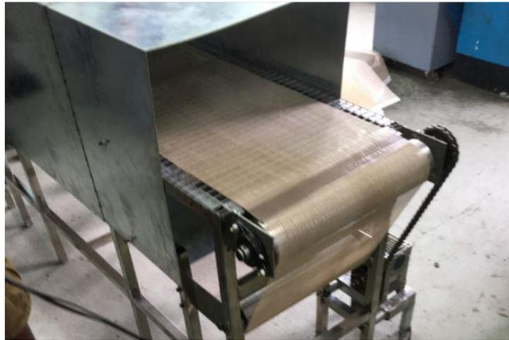
Figure 22: Enclosure Installed in Prototype
