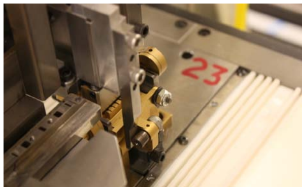
Figure 43: Linear cam and support mounted on transfer station
