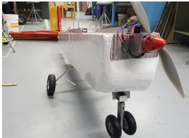
Figure 52: Completed nose with propulsion equipment installed.
