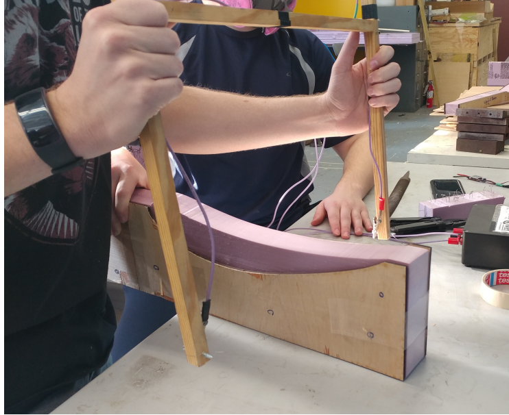
Figure 43: Hot wire cutting foam ribs using laser-cut wooden templates.
