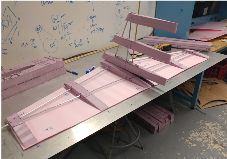
Figure 49: Horizontal and vertical tail frame assembly.
