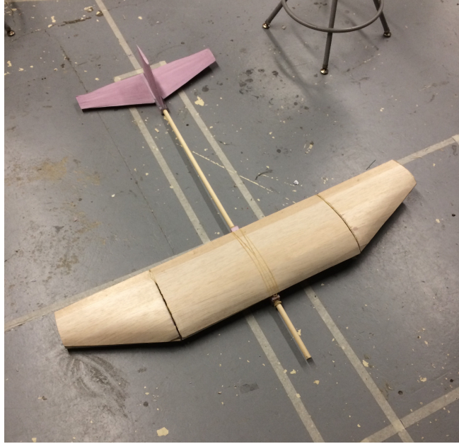
Figure 45: One-third scale glider model.
