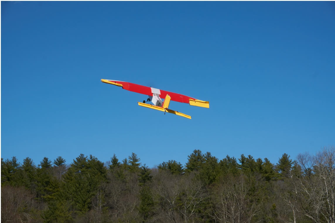
Figure 60: The aircraft in flight entering a stall condition.
