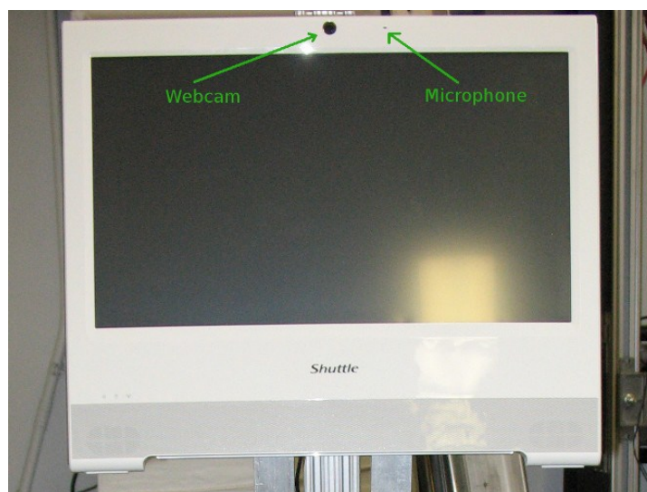
Figure 12: Webcam and microphone built into the robot's user interface computer
