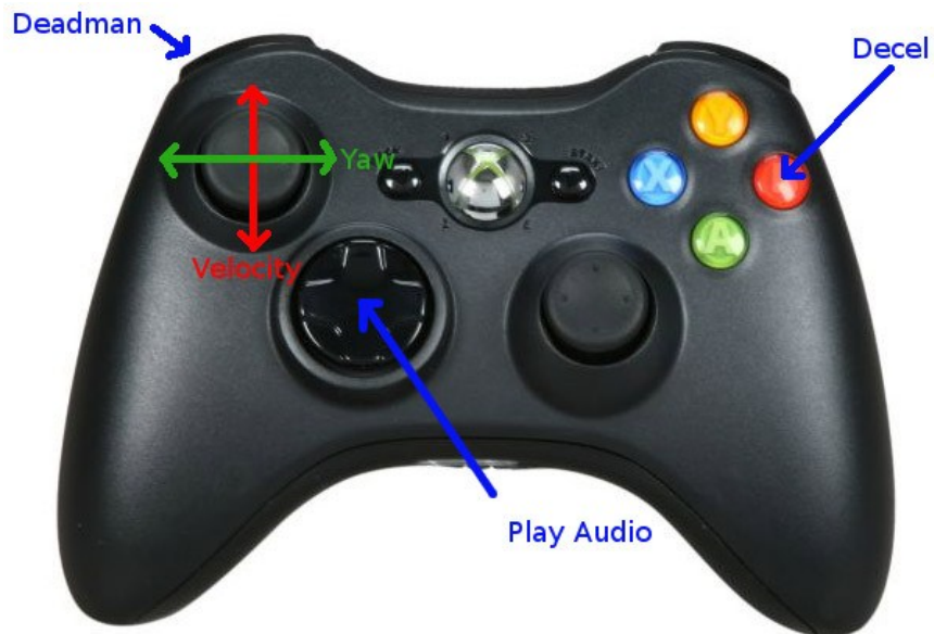
Figure 5: Xbox 360 controller button mappings for remote control of robot
