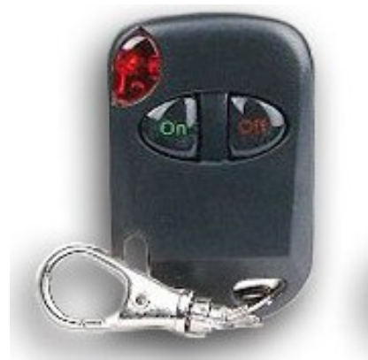
Figure 7: Wireless relay fob for robot emergency stop system
