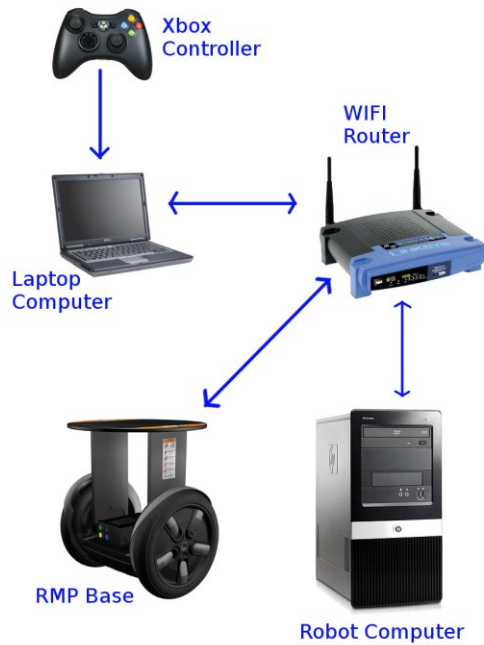
Figure 4: Network setup for remote control of robot
