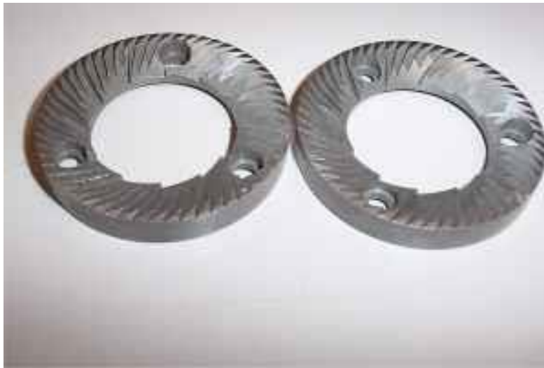
Figure 7: Flat Burr Grinder (Frew, 2007)
