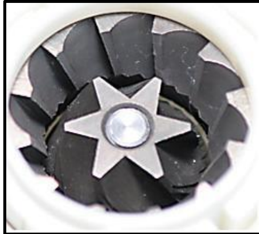
Figure 9: Burr Grinder ("Burr Grinder vs Blade Grinder – Which One Is The Best?," 2013)
