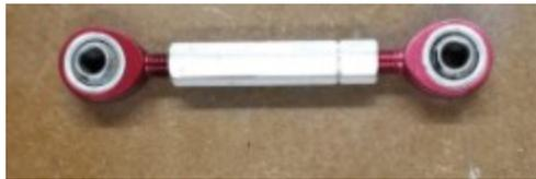
Figure 22. Ball Joint Rod Ends and Turnbuckle
