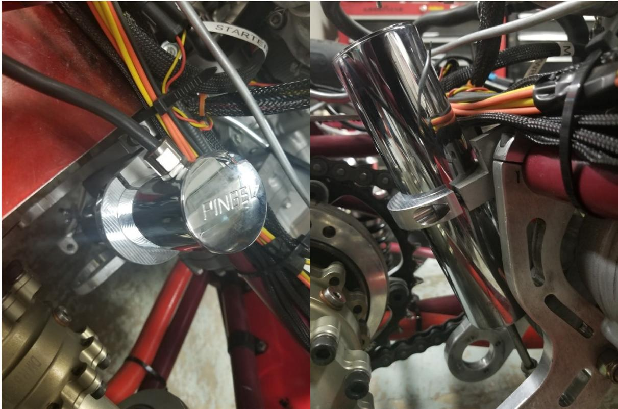
Figure 38. Pingel Electric Speed Shifter Mounted to Car
