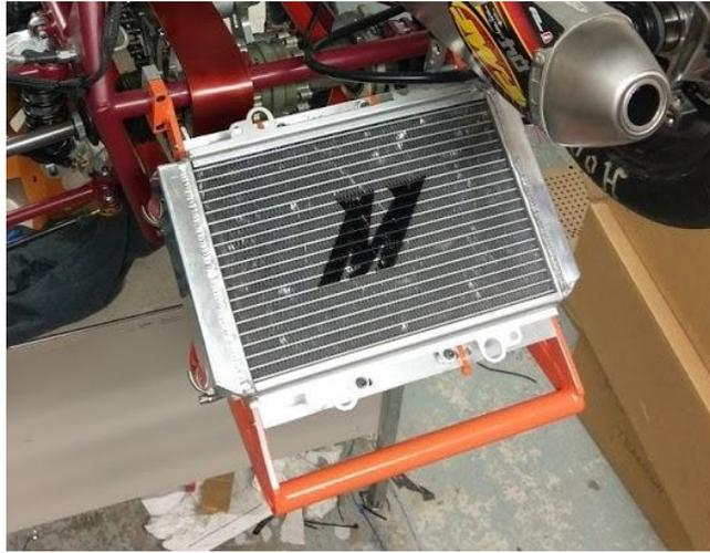
Figure 71. Radiator Mounted to Jack Point on Car
