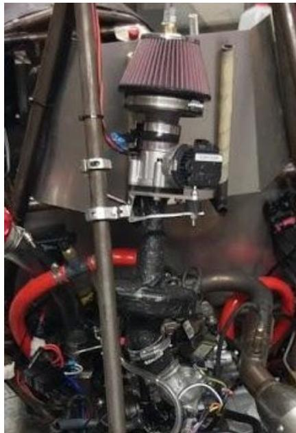
Figure 56. Intake Prototype Mounted in Car
