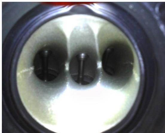
Figure 48. WR450F Integral Intake Runner Extension and Intake Valve Stems
