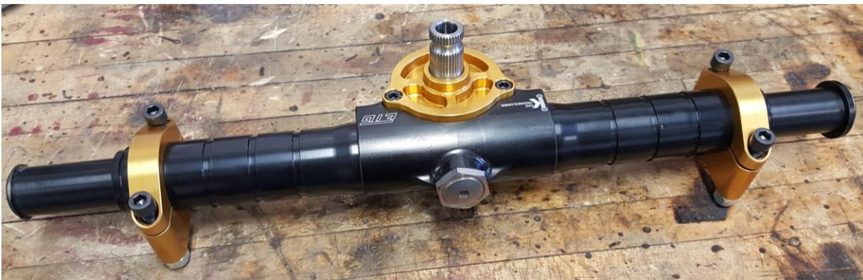
Figure 103. Kaz Technologies steering rack
