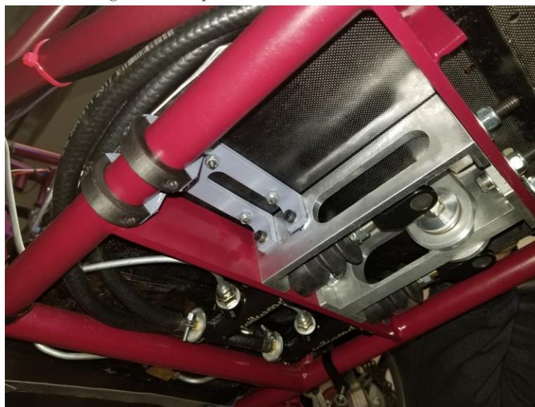
Figure 132. Bottom View of Mounted Throttle Pedal
