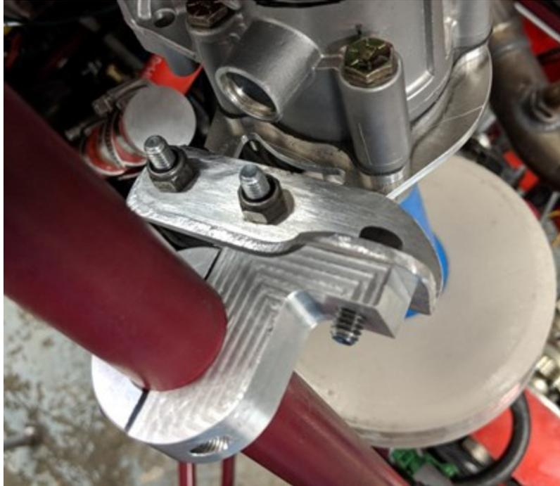
Figure 60. Top View of Upper Air Intake Mount to Frame
