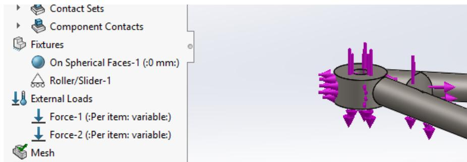
Figure 90. Forces applied to A-Arm
