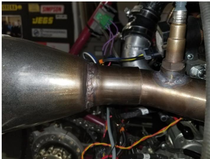
Figure 64. Exhaust Slip Fit
