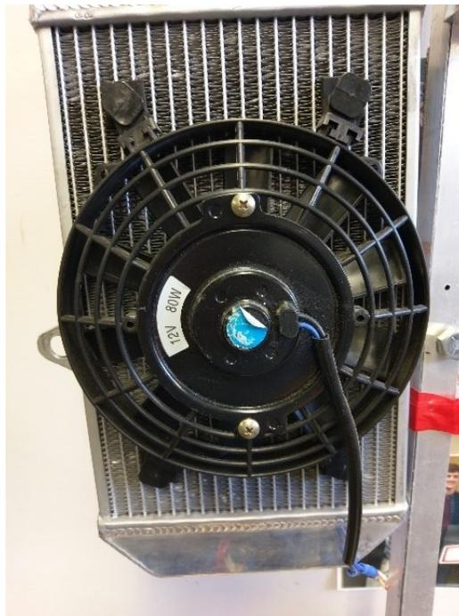
Figure 67. Test Bench Radiator and Fan
