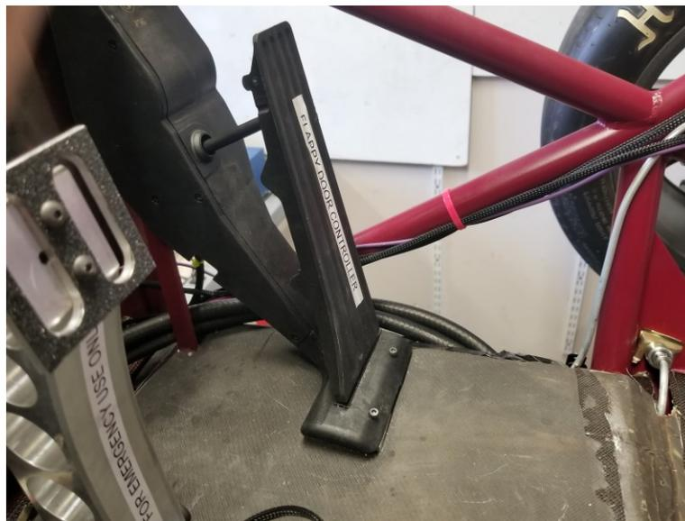
Figure 131. Top View of Mounted Throttle Pedal
