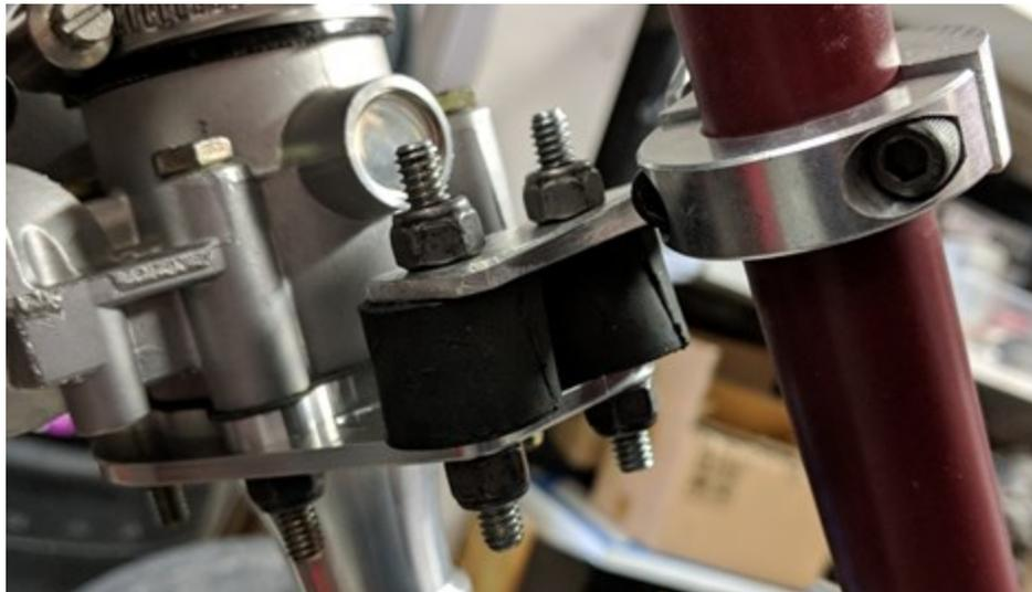
Figure 61. Side View of Upper Air Intake Mount to Frame – Throttle Body at Left, Main Roll Hoop Brace at Right
