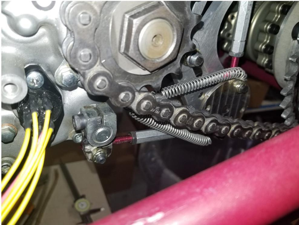
Figure 34. Shifting Mechanism return Springs
