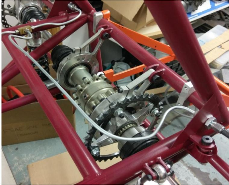
Figure 10. Completed Differential Mounts in Frame
