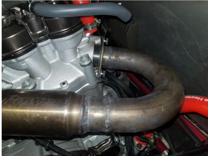
Figure 63. Header Pipe Modification
