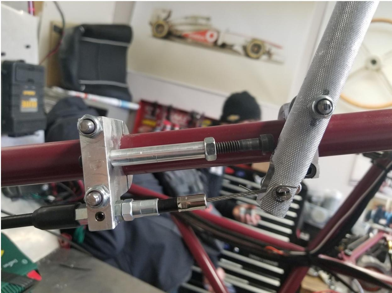
Figure 32. Hand Clutch Assembly
