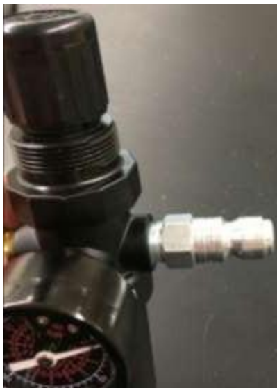
Figure 43: Male quick disconnect of regulator that interfaces with compressed airline
