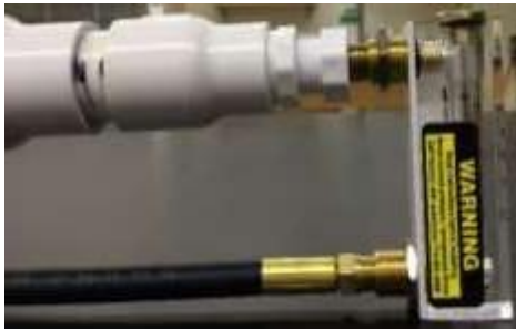
Figure 38: threaded nipple and airline hose attached to rotameter
