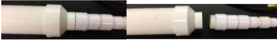
Figure 36: A) reducers attached; Figure 37: B) Reducers unattached from reducing coupling
