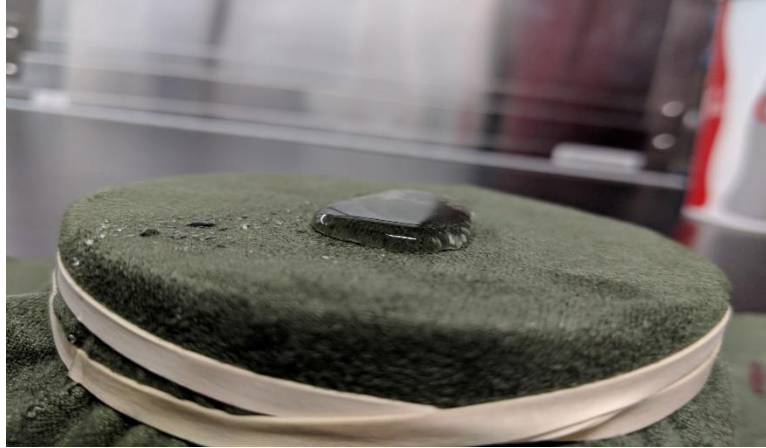
Figure 16: Neoprene Hydrophobicity Test
