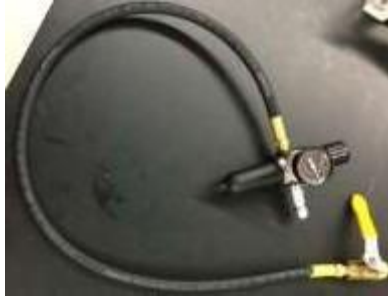
Figure 40: Ball valve connected to regulator via airline hose
