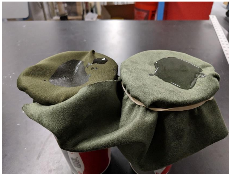
Figure 17: Hydrophobicity Test after 5 Minutes
