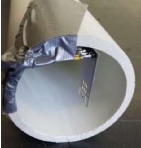
Figure 44: Rev C sensor secured at end of wind tunnel
