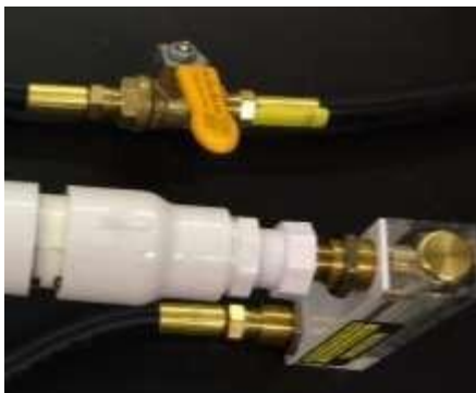
Figure 39: Ball valve attached to rotameter via airline hose
