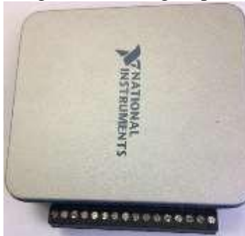
Figure 46: DAQ box used with the system; wires insert into the side below screws
