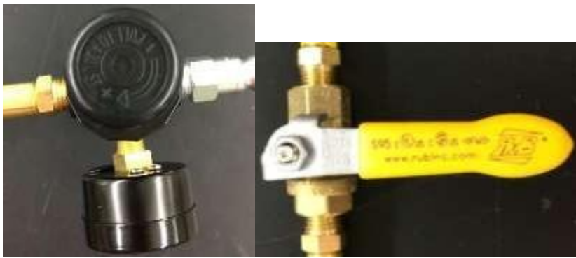
Figure 41: A) Regulator in closed position; Figure 42: B) Ball valve in closed position
