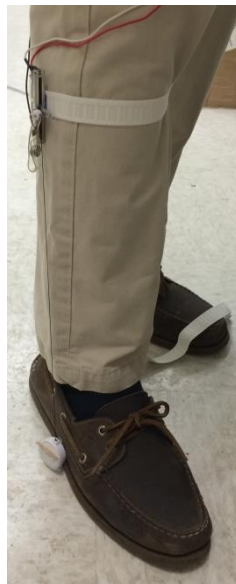
Figure 39: Linear Potentiometer attached to the calf of a test subject.
