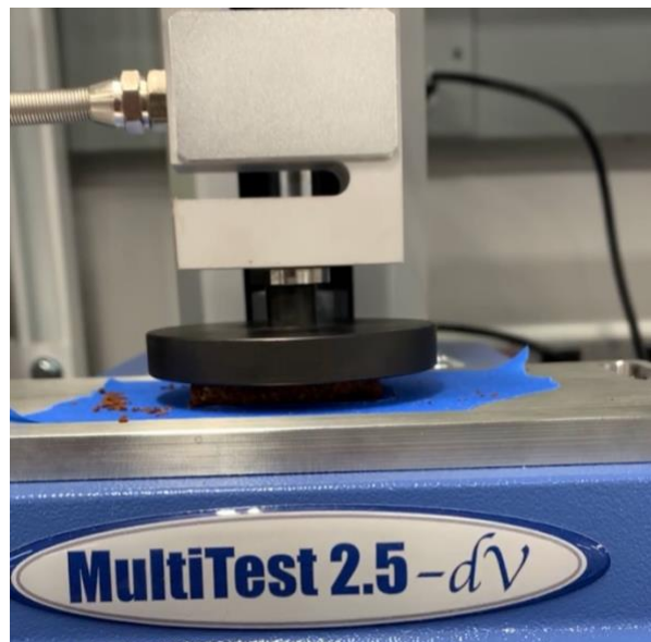
Figure 4. Compression test on a sample post processed at 300°F for 18 minutes.
