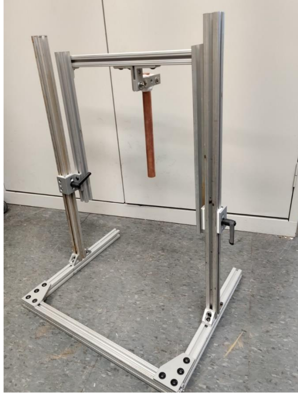
Figure A1. 5: Quick adjustable frame for holding the copper rod.
