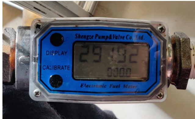
Figure A1. 3: The flow meter used in the used in the turbulence generation system.
