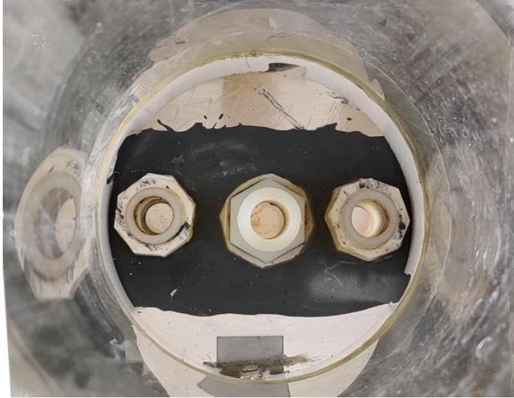
Figure A1. 1: Top view of the turbulence generation system bottom.
