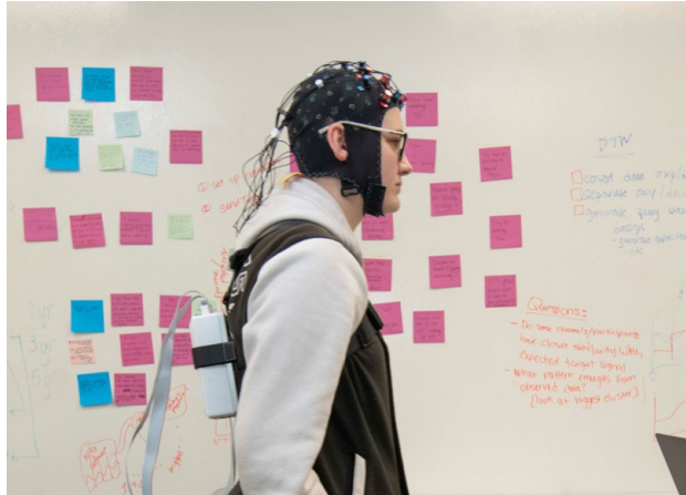
Figure 4: fNIRS device on a patient. The device includes the cap, sensors, and a small portable computer
