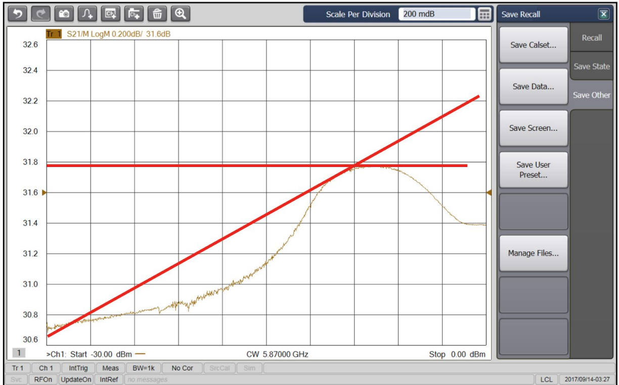
Figure 12: S21 power sweep of the modified amplifier. As seen in this graph the amplifier only makes 31 dBm of power before going into its P1 dB compression point around 31.8 dBm and is no longer linear.
