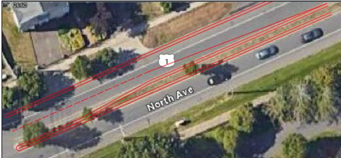
Figure 34. Images of potential left turn storage lane adjustment to existing median on North Ave. westbound.
