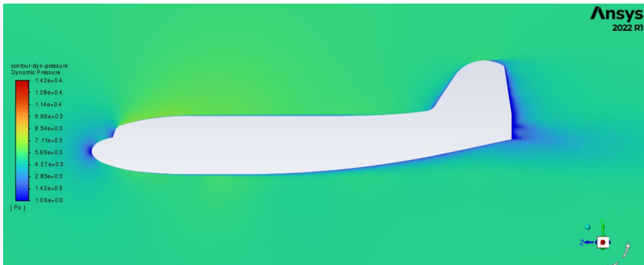
Figure 32: Dynamic Pressure Distribution Around DC-3 Centerline
