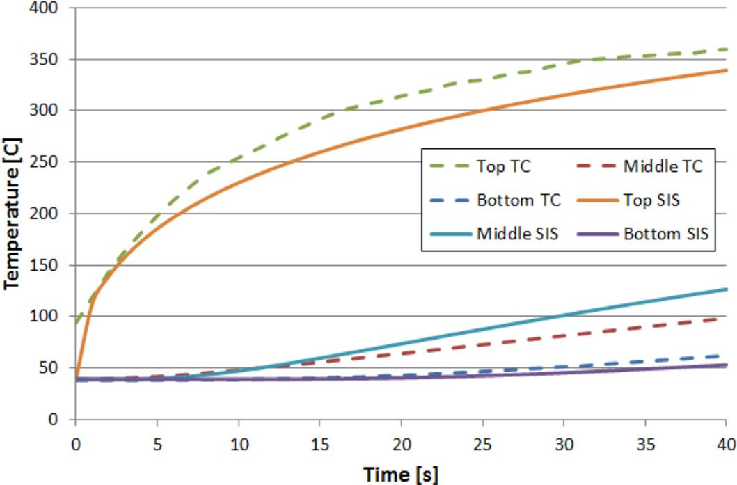
Figure 4.5.1: Boundary Condition 1 Temperature Distribution (SIS stands for Semi-Infinite Solid)
