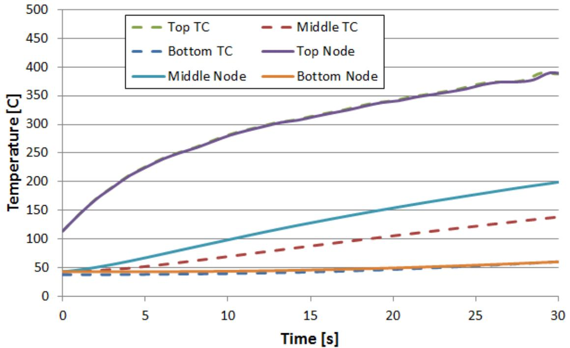
Figure 4.5.3: Boundary Condition 2 Temperature Distribution
