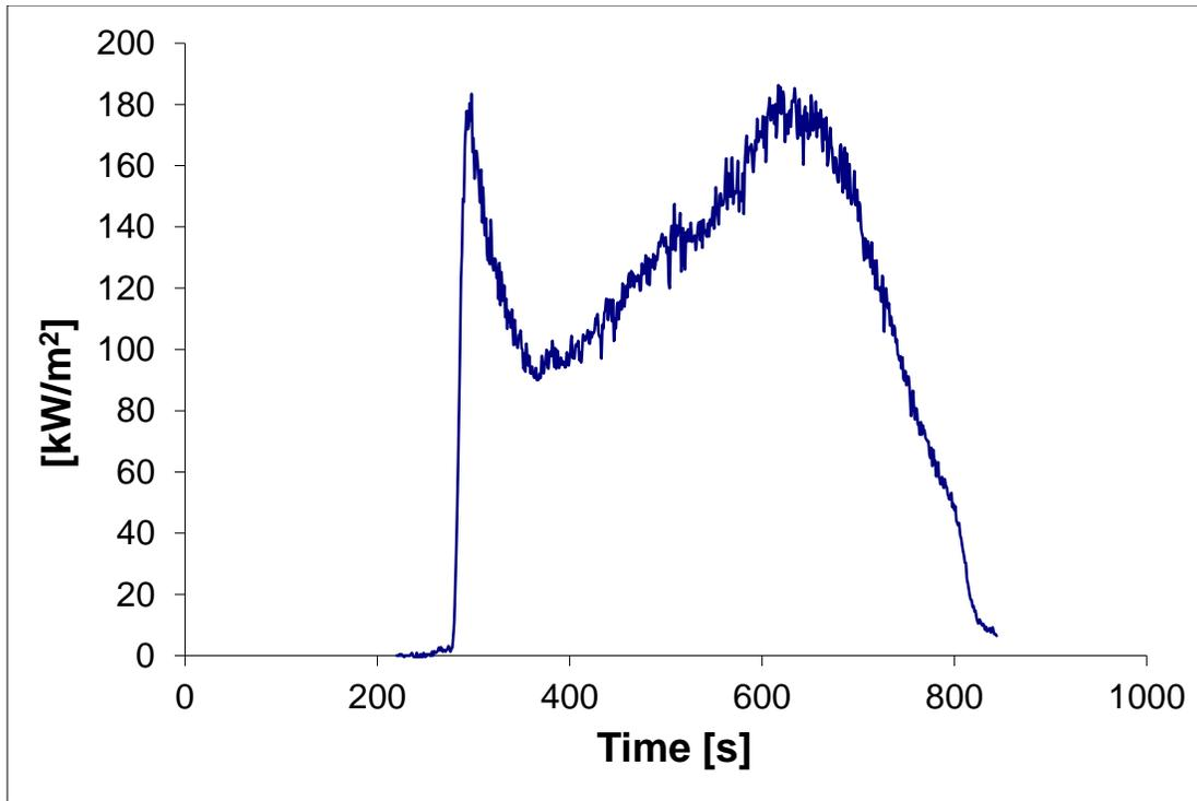
Figure 13: Heat Release Rate per Unit Area CP 702, Test 2
