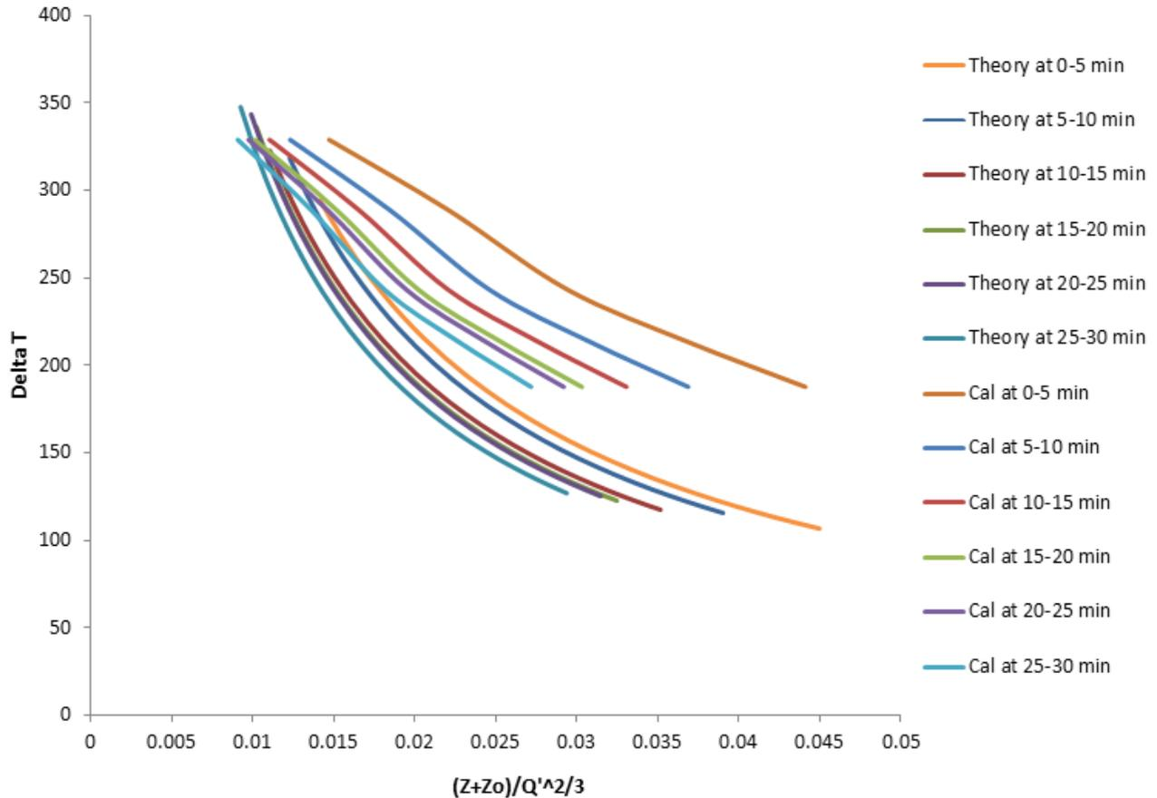
Figure 5: Graphical results of calculated theory compared to actual calibration data using plume mass flow rate equation (8a).
