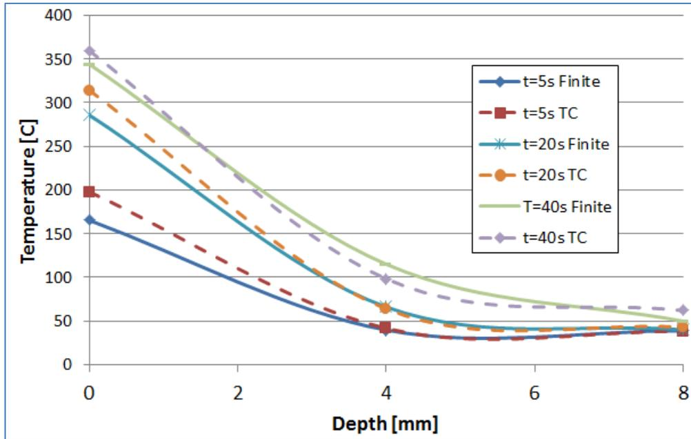
Figure 3.4.6: Temperature Profile for Kreysler System 1, BC-3
