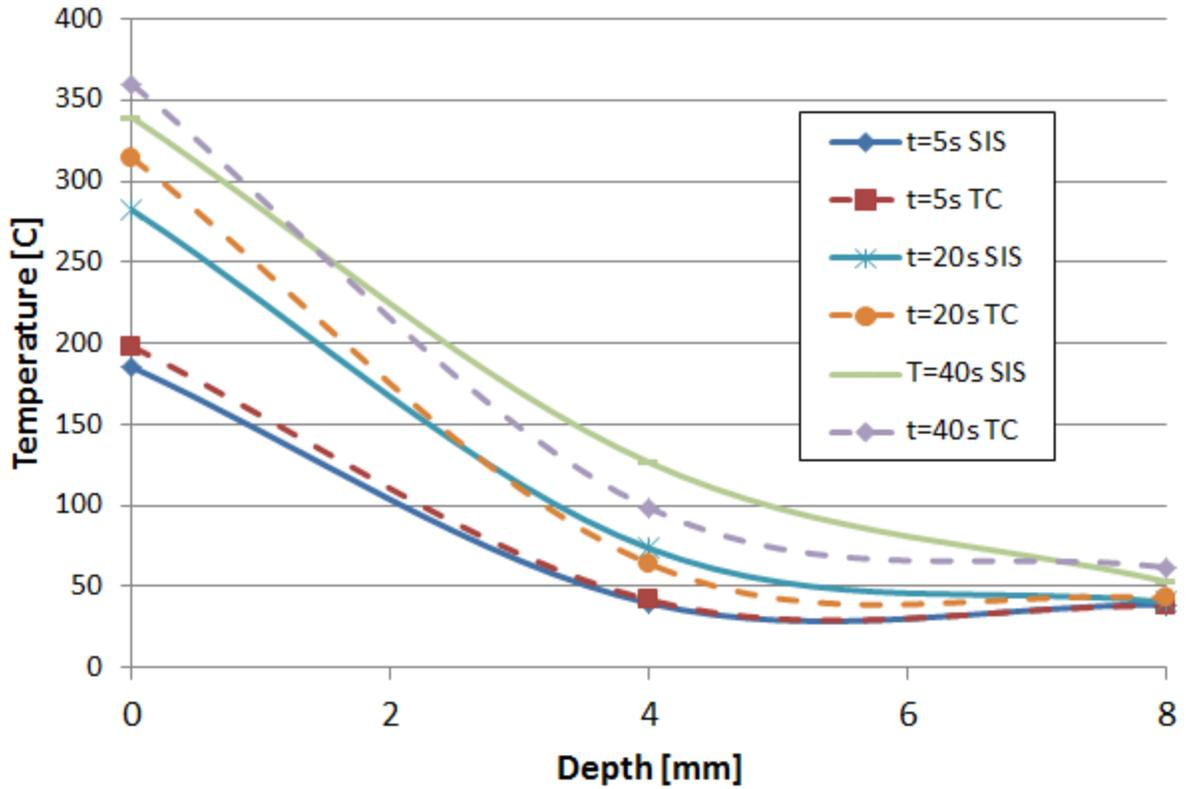
Figure 4.5.2: Boundary Condition 1 Temperature Profile (SIS stands for Semi-Infinite Solid)
