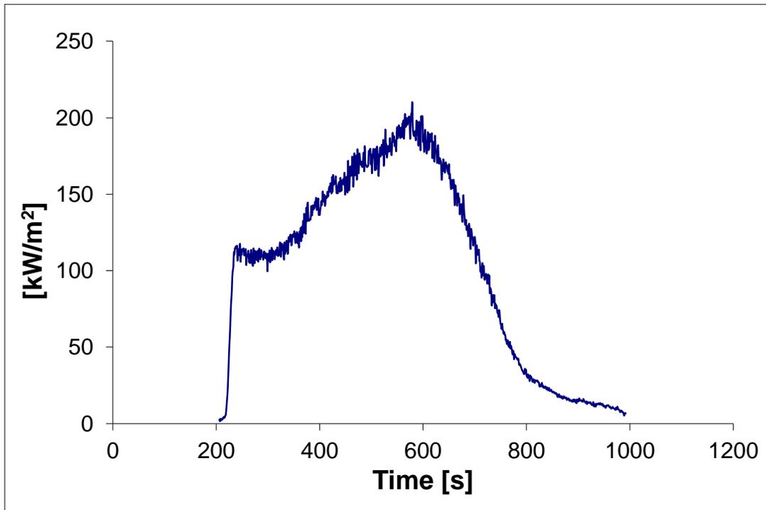
Figure 10: Heat Release Rate per Unit Area CP 802, Test 1
