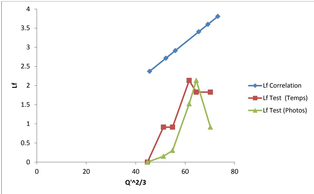
Figure 2: Theoretically calculated flame heights and test flame heights based on test temperature data and visual data from test report.
