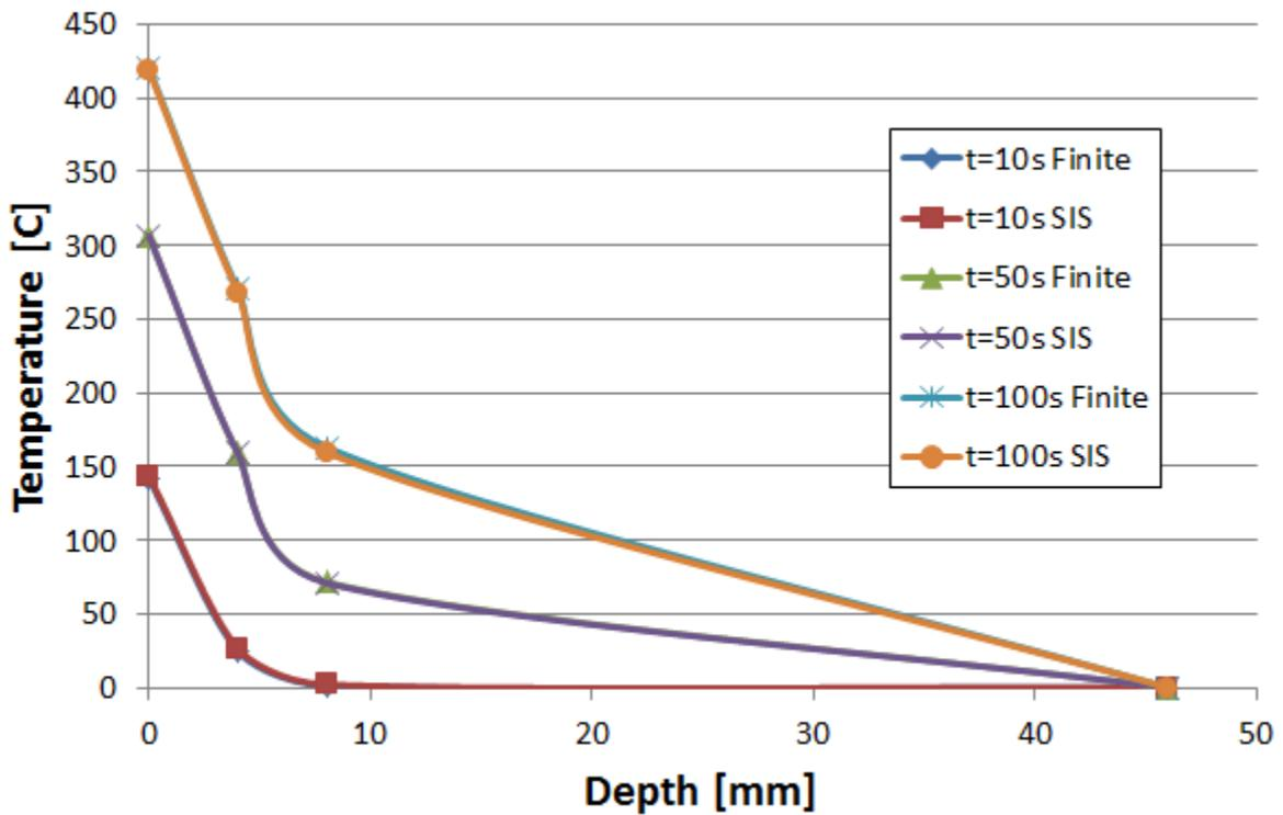
Figure 2.4.2: Temperature Profile for Model Verification (SIS stands for Semi-Infinite Solid)
