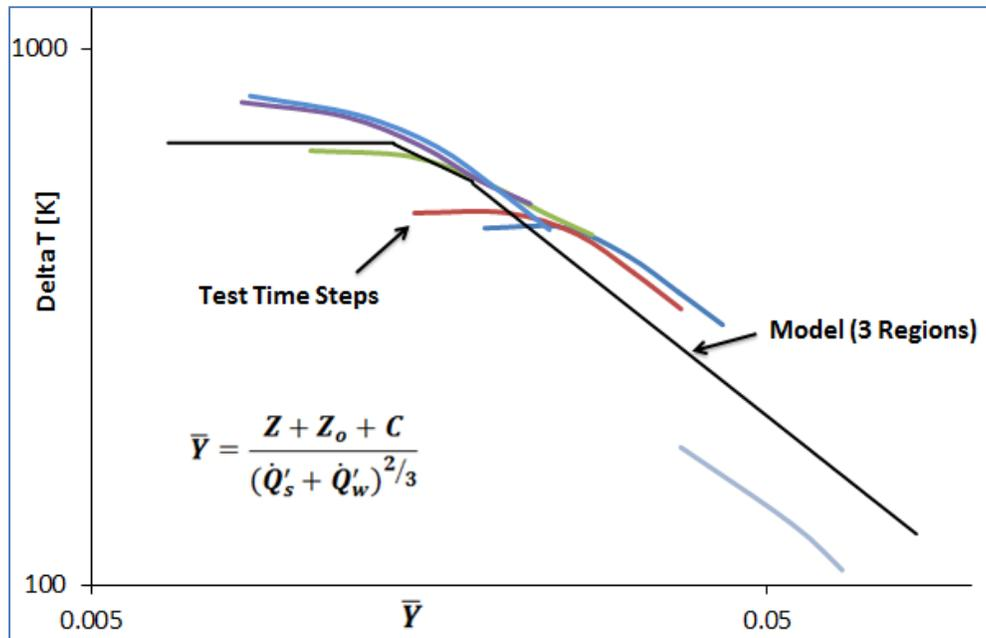
**Figure 4.2.3: The final model created for the NFPA 285 test, as well as the data recorded for the 6 time steps during the test.**
