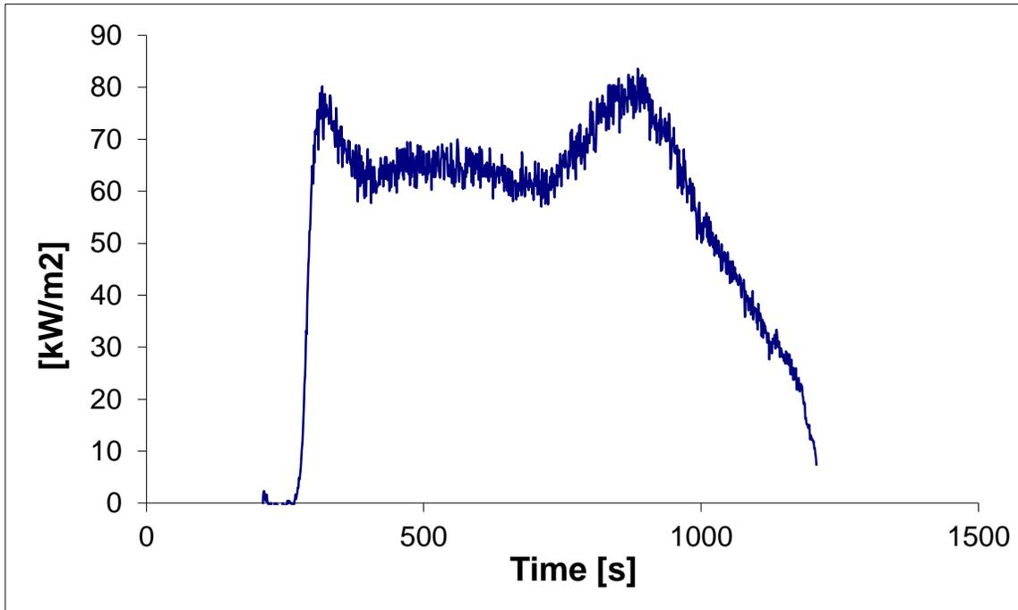
Figure 6: Heat Release Rate per Unit Area Kreysler 1, Test 1
