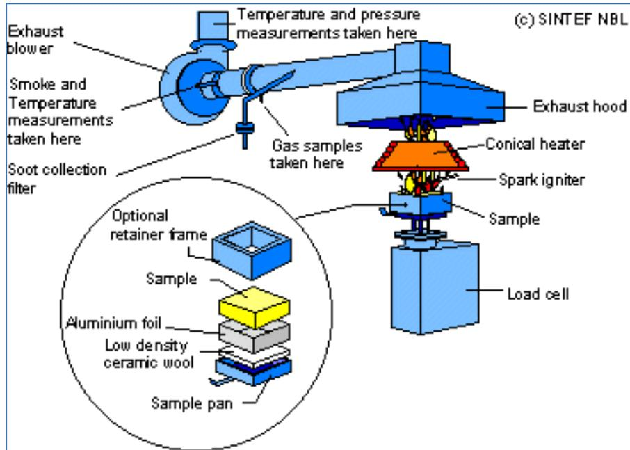
Figure 2.1.1: Diagram of Cone Calorimeter (SINTEF).
