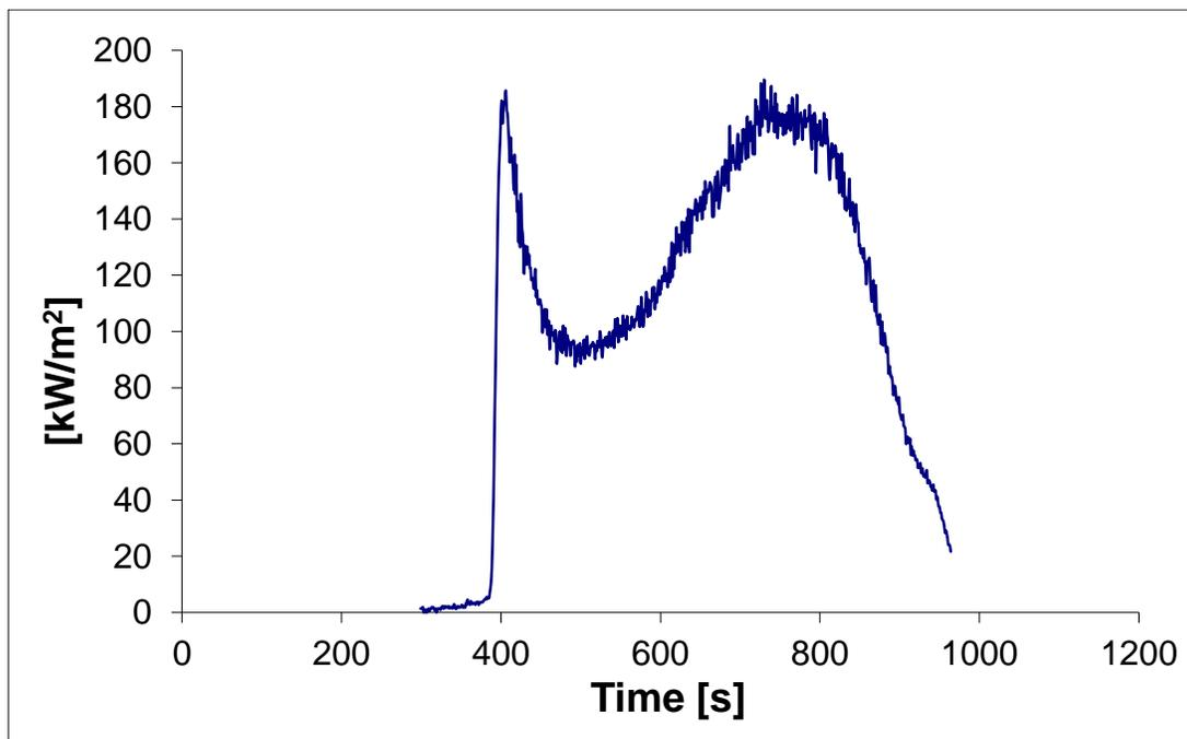
Figure 12: Heat Release Rate per Unit Area CP 702, Test 1
