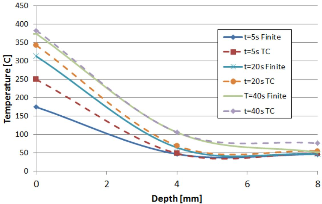
Figure 4.2.6: Boundary Condition 3 Temperature Profile
