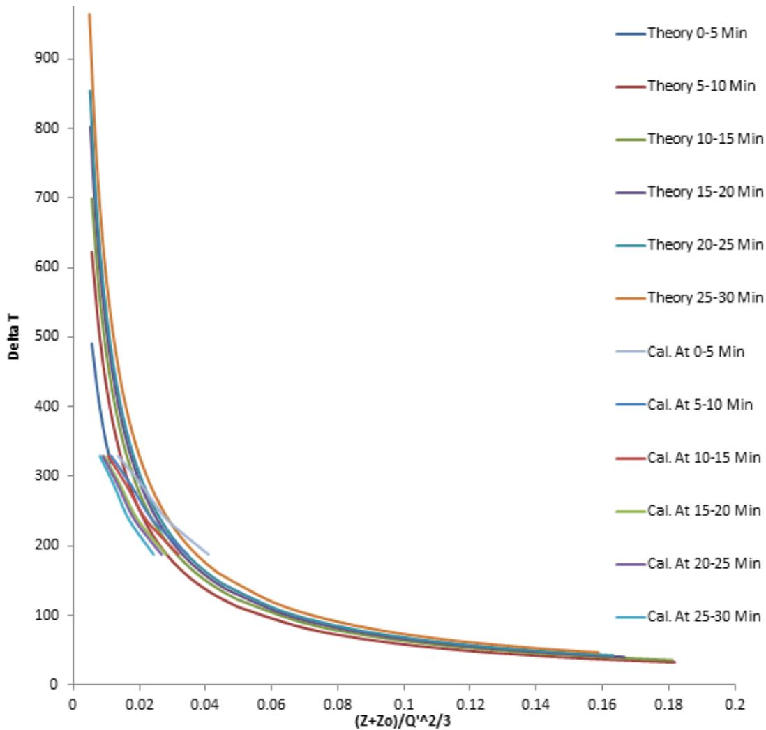
Figure 3: Graphical results of calculated theory compared to actual calibration data using plume mass flow rate equation (6a).
