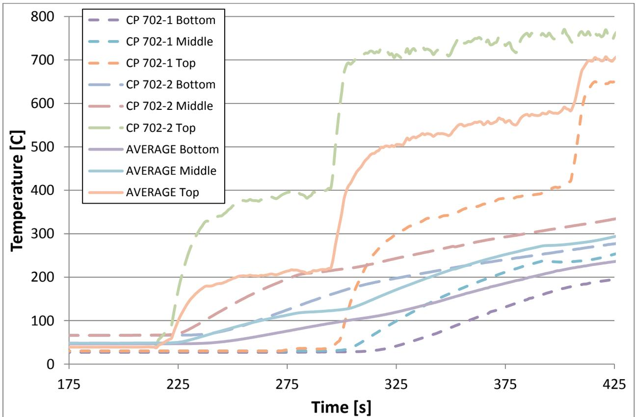
Creative Pultrusion      Skin 702      Test 1      50 kW/m<sup>2</sup>      10-25\_Sample3-1\_702\_50kW.txt
