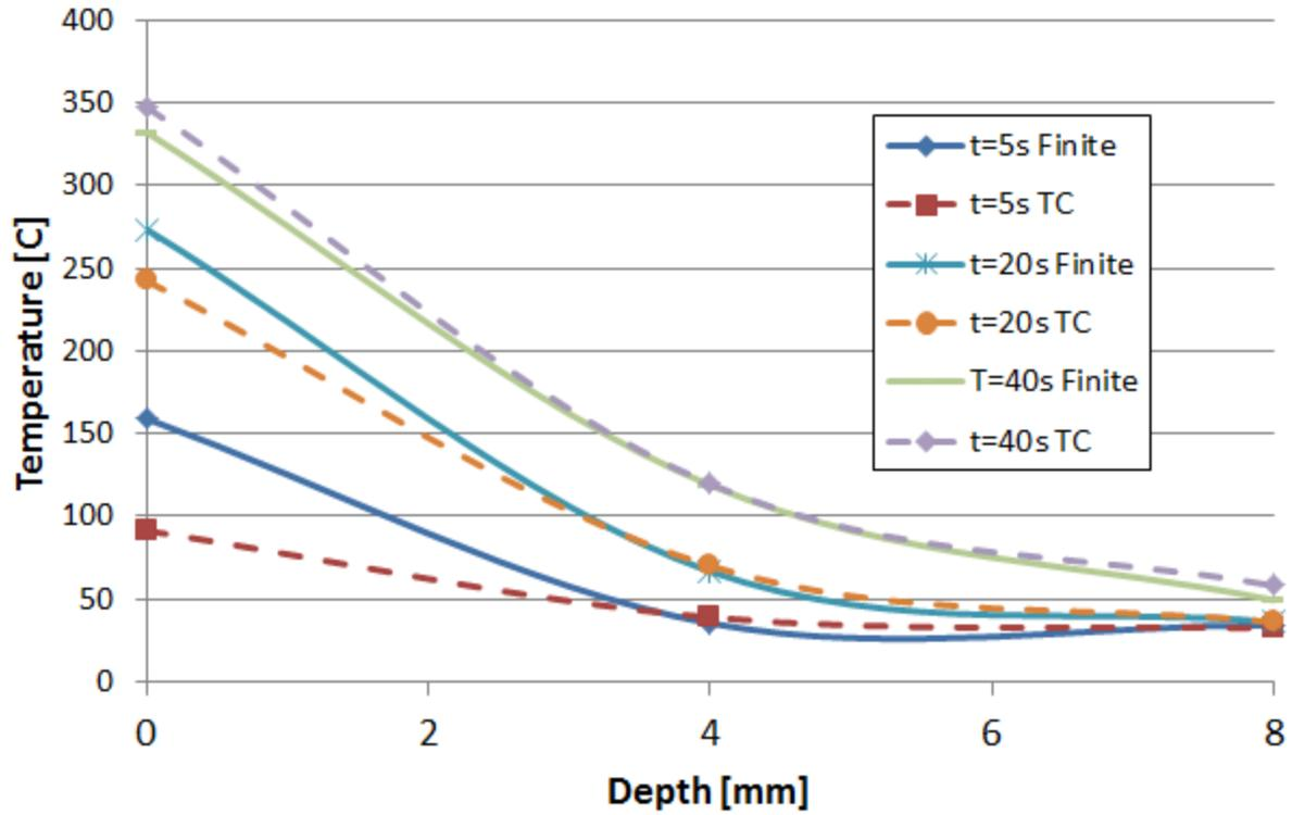
Figure 4.3.6: Boundary Condition 3 Temperature Profile
