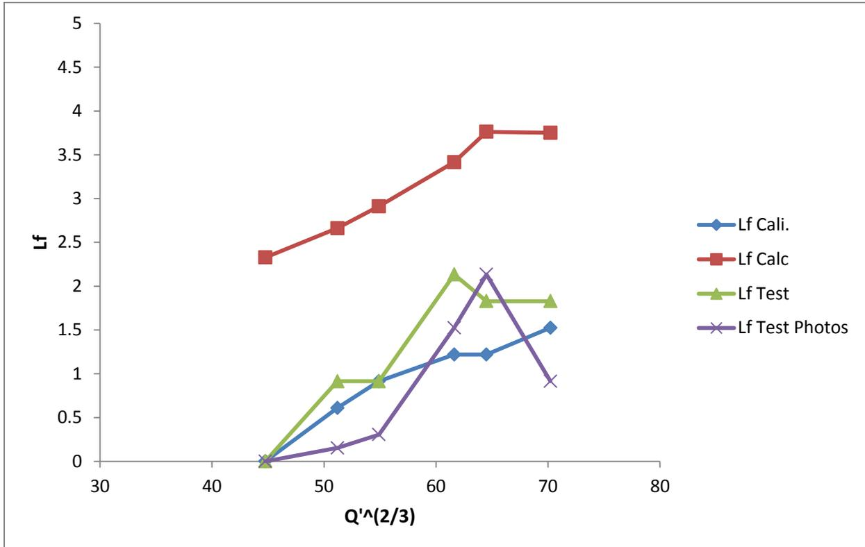
Figure 1: Theoretically calculated flame heights, actual calibration and test flame heights based on temperature and visual data from test report.
