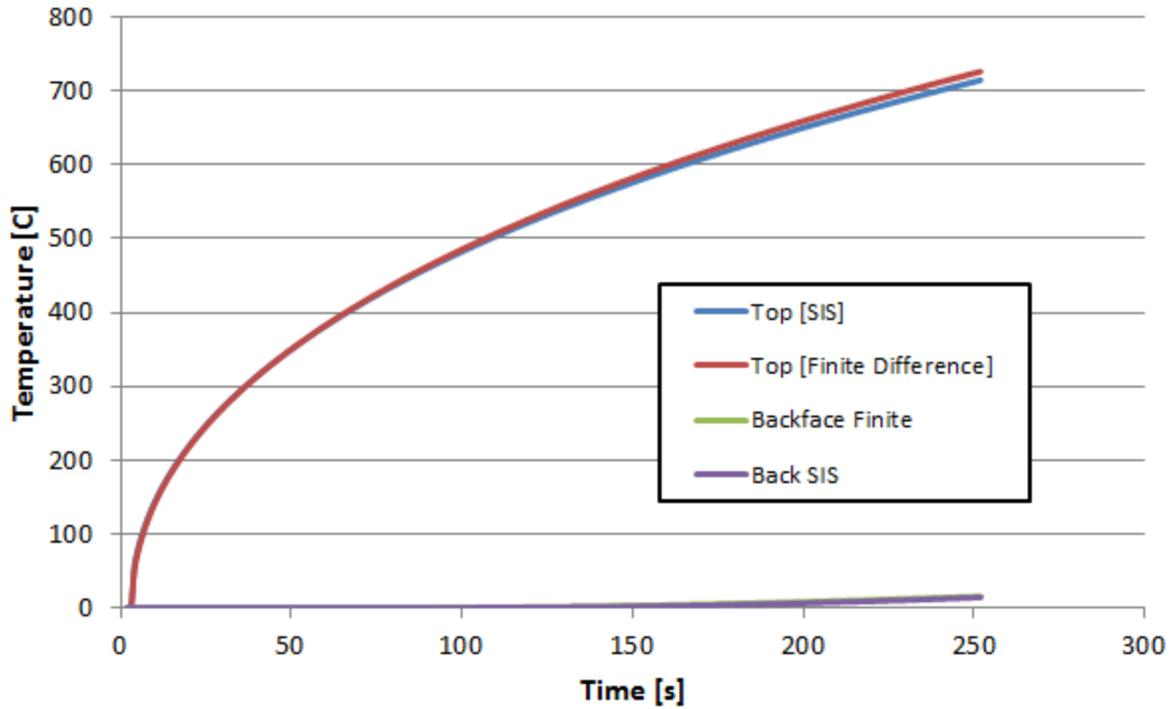
Figure 2.4.1: Temperature Distribution for Model Verification (SIS stands for Semi-Infinite Solid)
