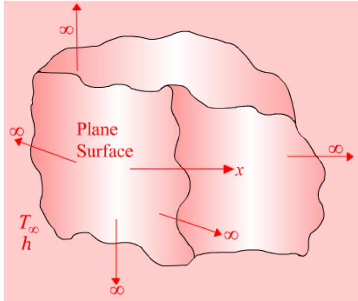
Figure 2.1.1: Schematic of a Semi -Infinite Body (ECourses, Transient Heat Conduction in Semi-Infinite Solids)
