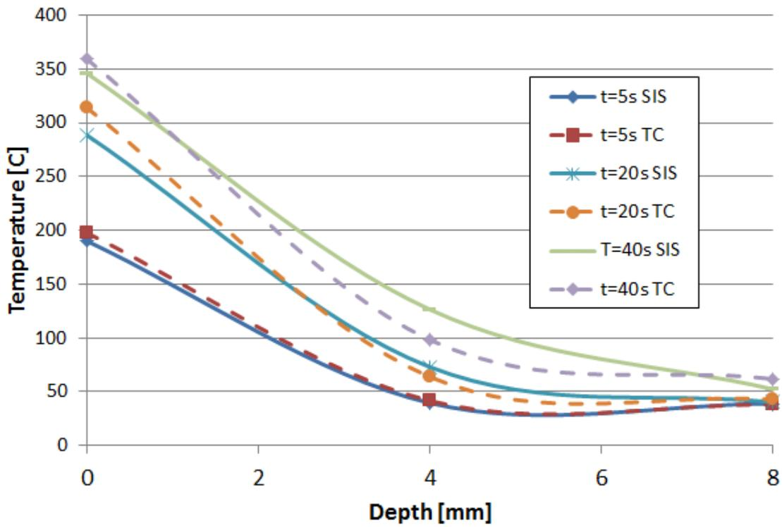
Figure 4.4.2: Boundary Condition 1 Temperature Profile (SIS stands for Semi-Infinite Solid)
