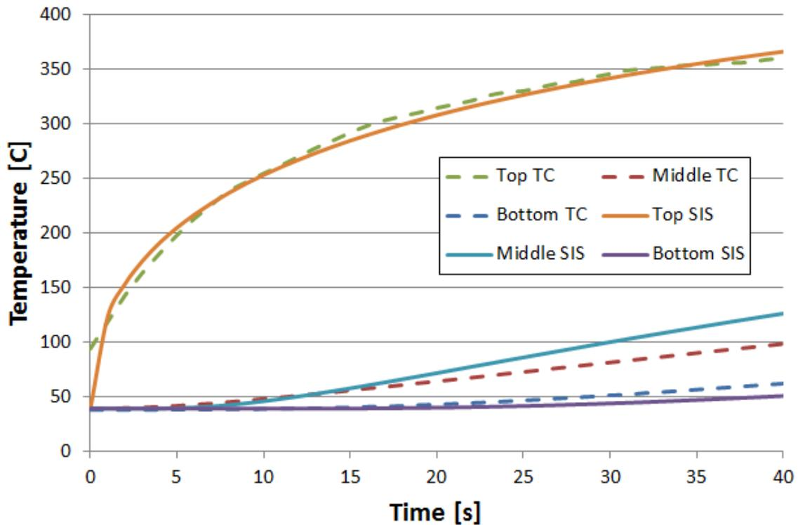
**Figure 4.1.1: Boundary Condition 1 Temperature Distribution (SIS stands for Semi-Infinite Solid)**
