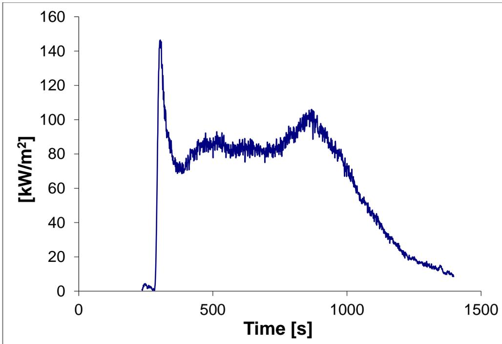
Figure 9: Heat Release Rate per Unit Area Kreysler 2, Test 2
