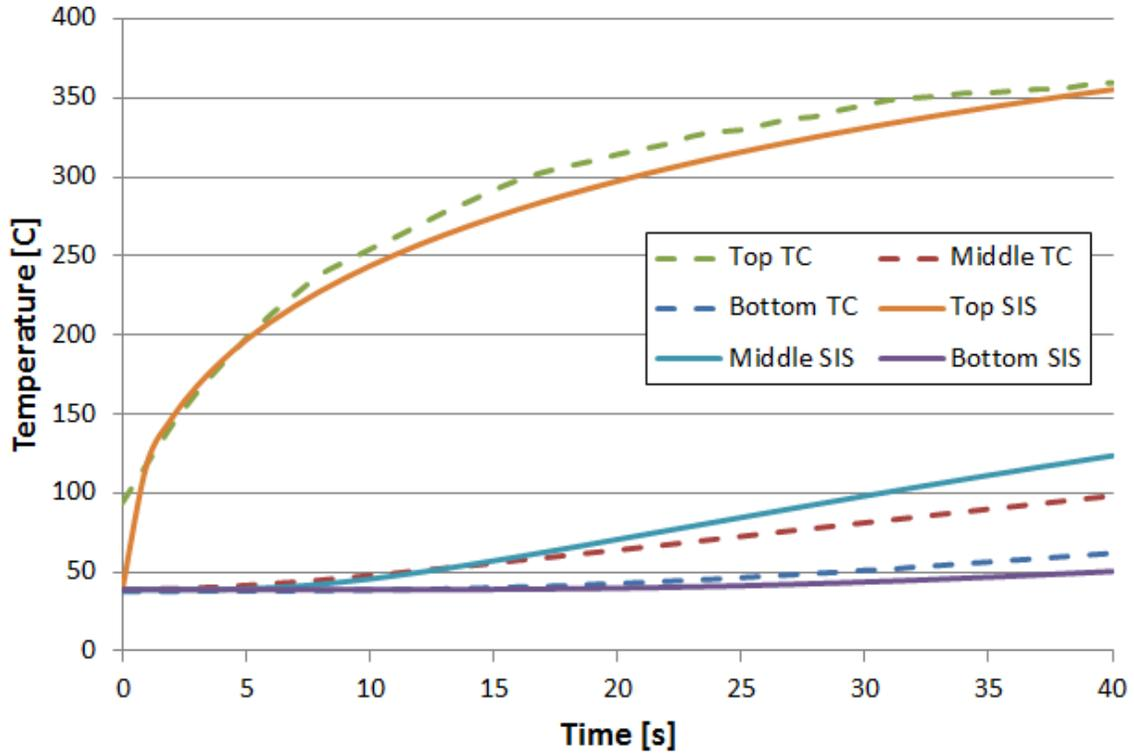
Figure 4.3.1: Boundary Condition 1 Temperature Distribution (SIS stands for Semi-Infinite Solid)
