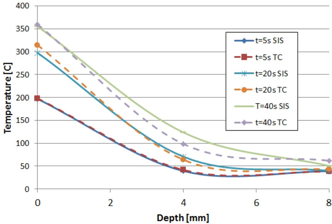
Figure 4.3.2: Boundary Condition 1 Temperature Profile (SIS stands for Semi-Infinite Solid)
