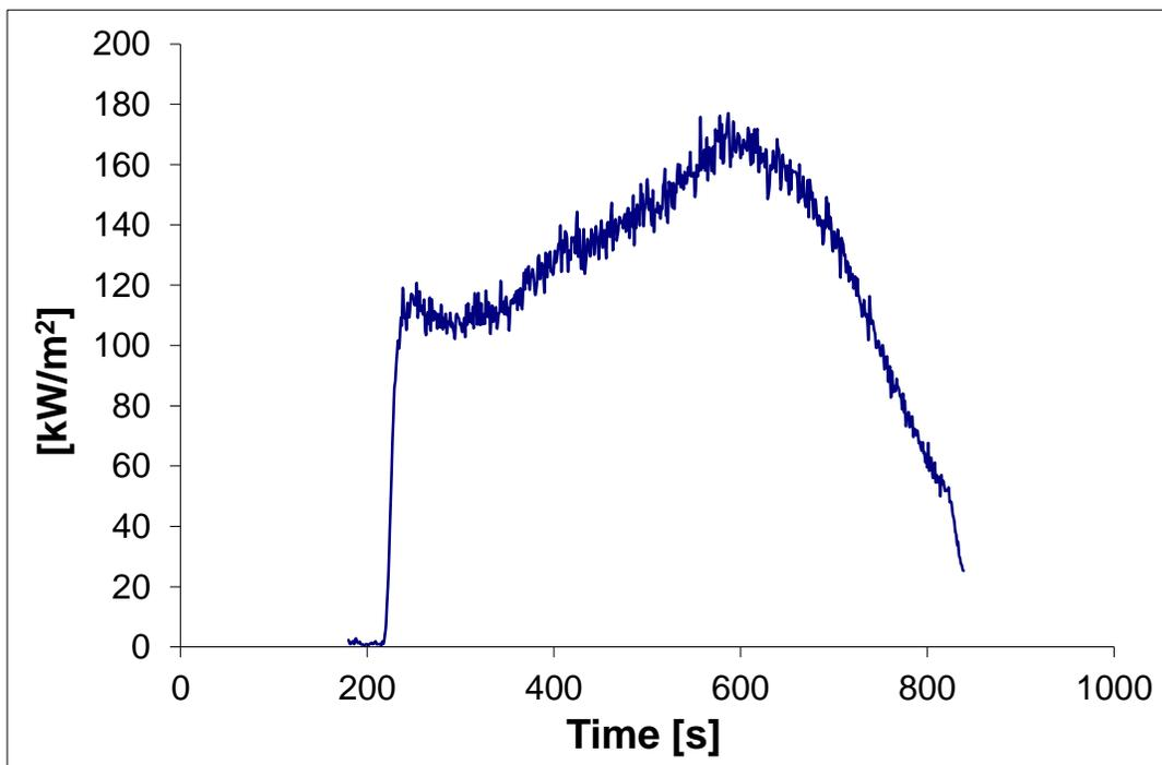
Figure 11: Heat Release Rate per Unit Area CP 802, Test 2
