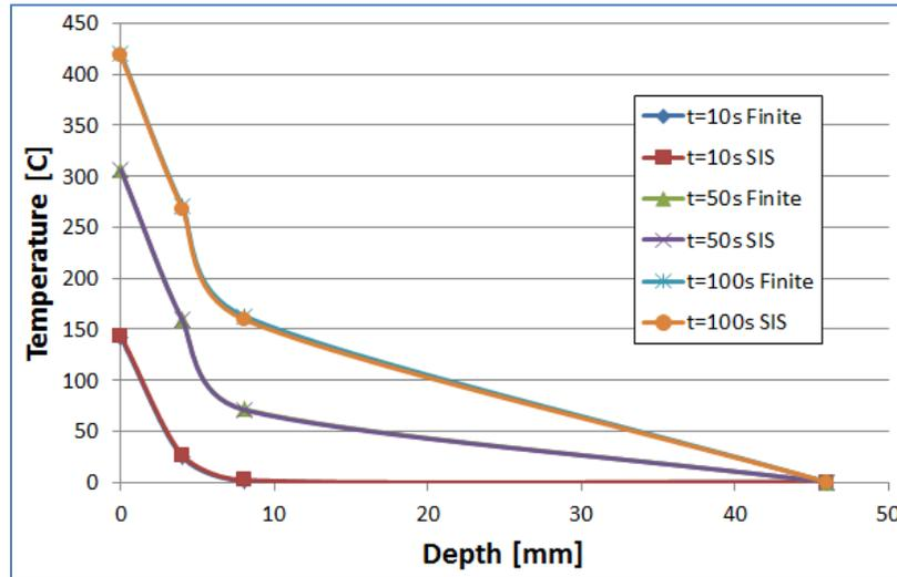
Figure 3.2.2: Temperature Profile for Model Verification (SIS stands for Semi-Infinite Solid)
