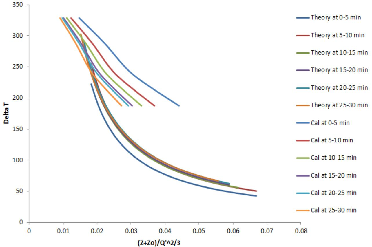
Figure 4: Graphical results of calculated theory compared to actual calibration data using plume mass flow rate equation (7a).
