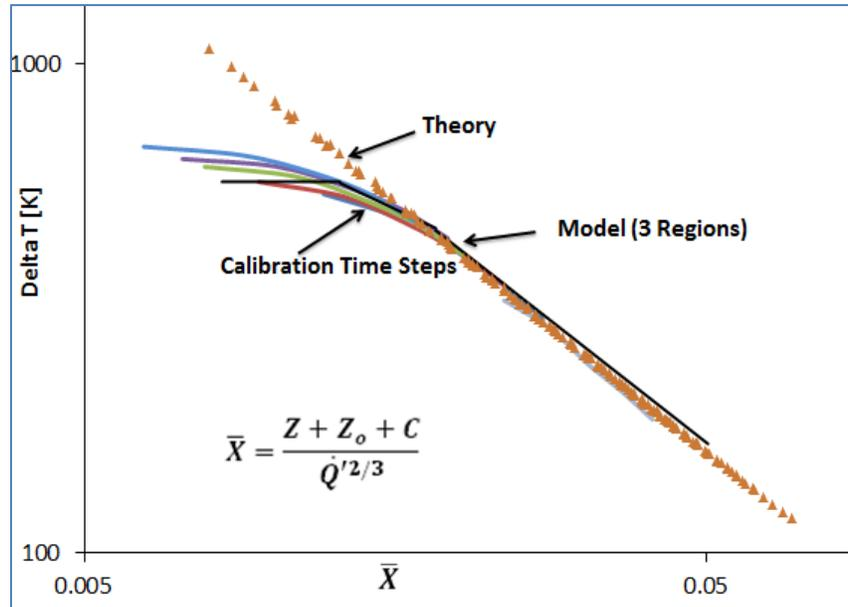
Figure 4.1.3: The final model created for the calibration of the NFPA 285 test, as well as the data for the 6 time steps and the calculated theory line.
