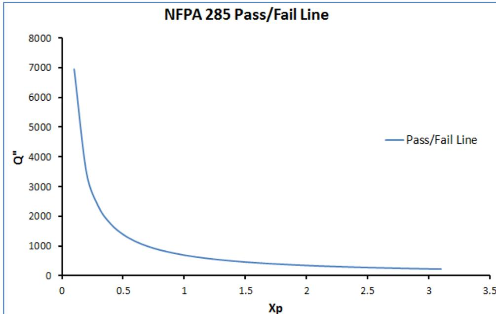
Figure 4.4.14: This graph demonstrates the prescriptive tool created to show the pass/fail curve for the NFPA 285 test. All combinations of  $Q''$  and  $x_p$  that fall below the curve indicate that the material would meet the acceptance criteria of NFPA 285, while pairs falling above the curve are not likely to comply.
