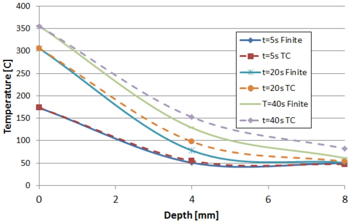
Figure 4.4.4: Boundary Condition 2 Temperature Profile
