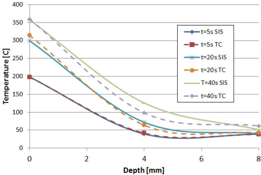
Figure 4.2.2: Boundary Condition 1 Temperature Profile (SIS stands for Semi-Infinite Solid)
