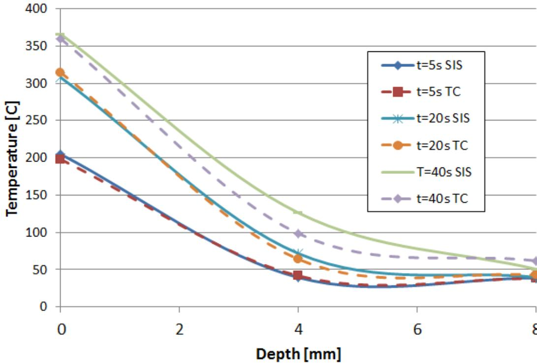
Figure 4.1.2: Boundary Condition 1 Temperature Profile (SIS stands for Semi-Infinite Solid)
