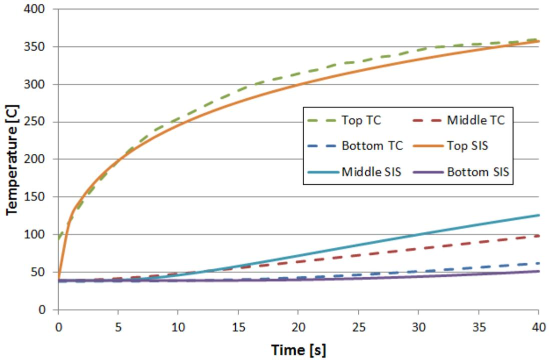
Figure 4.2.1: Boundary Condition 1 Temperature Distribution (SIS stands for Semi-Infinite Solid)
