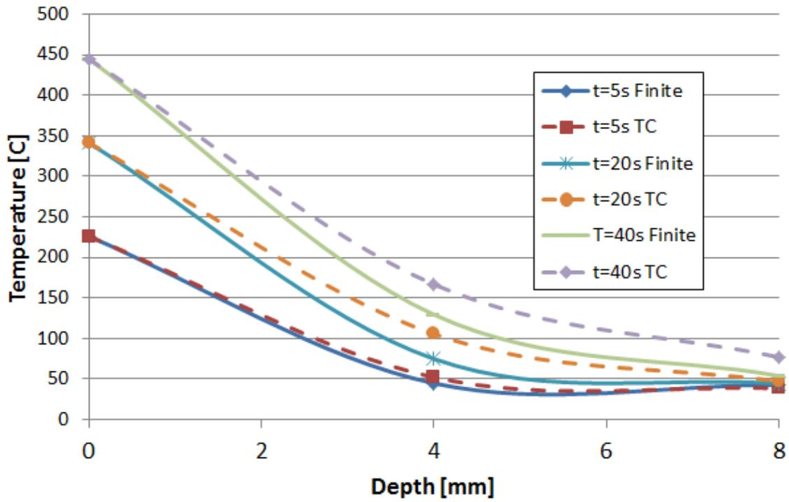
Figure 4.5.4: Boundary Condition 2 Temperature Profile
