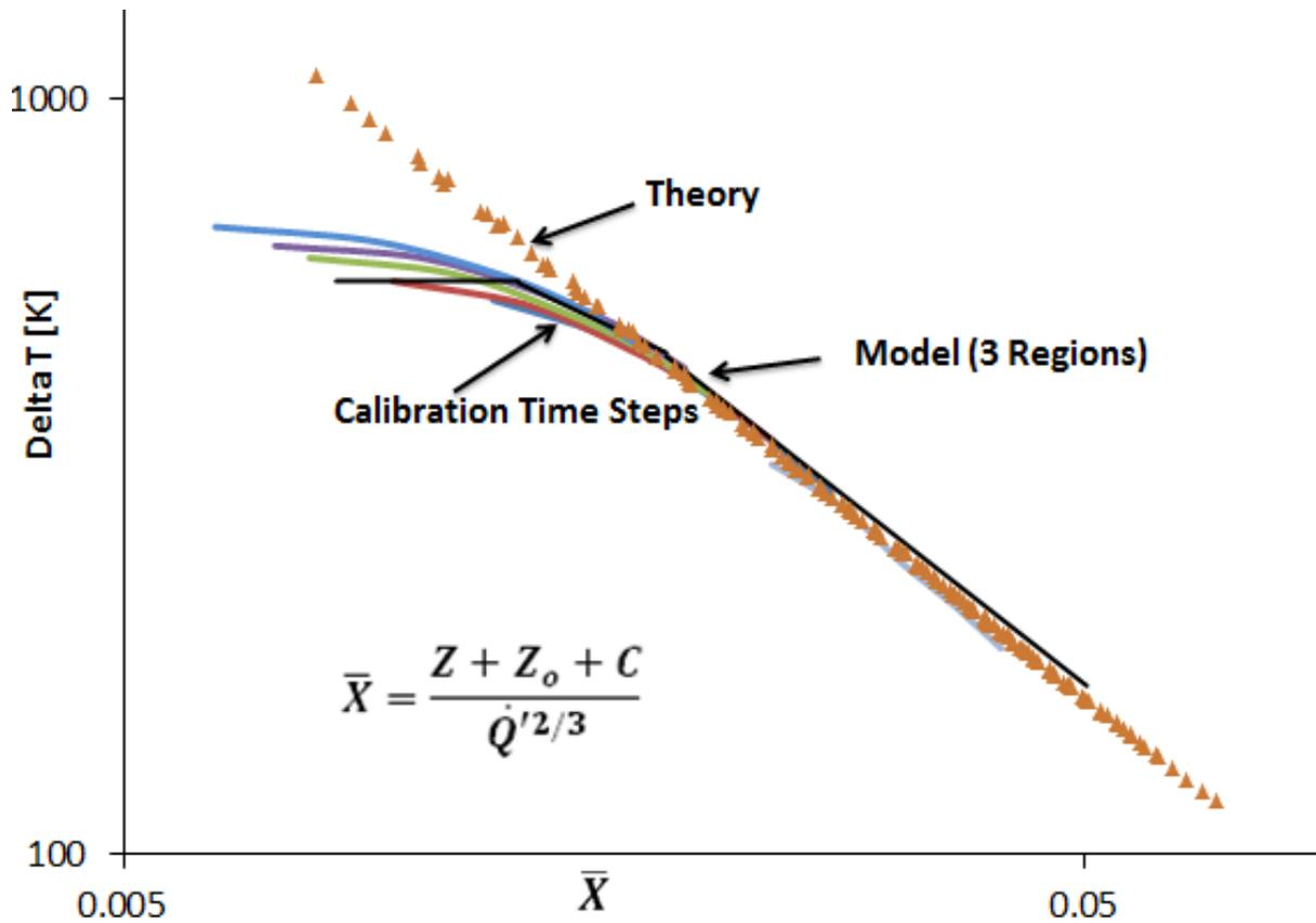
Figure 6: Graph comparing the theoretically calculated results, calibration data, and calibration model that was developed.
