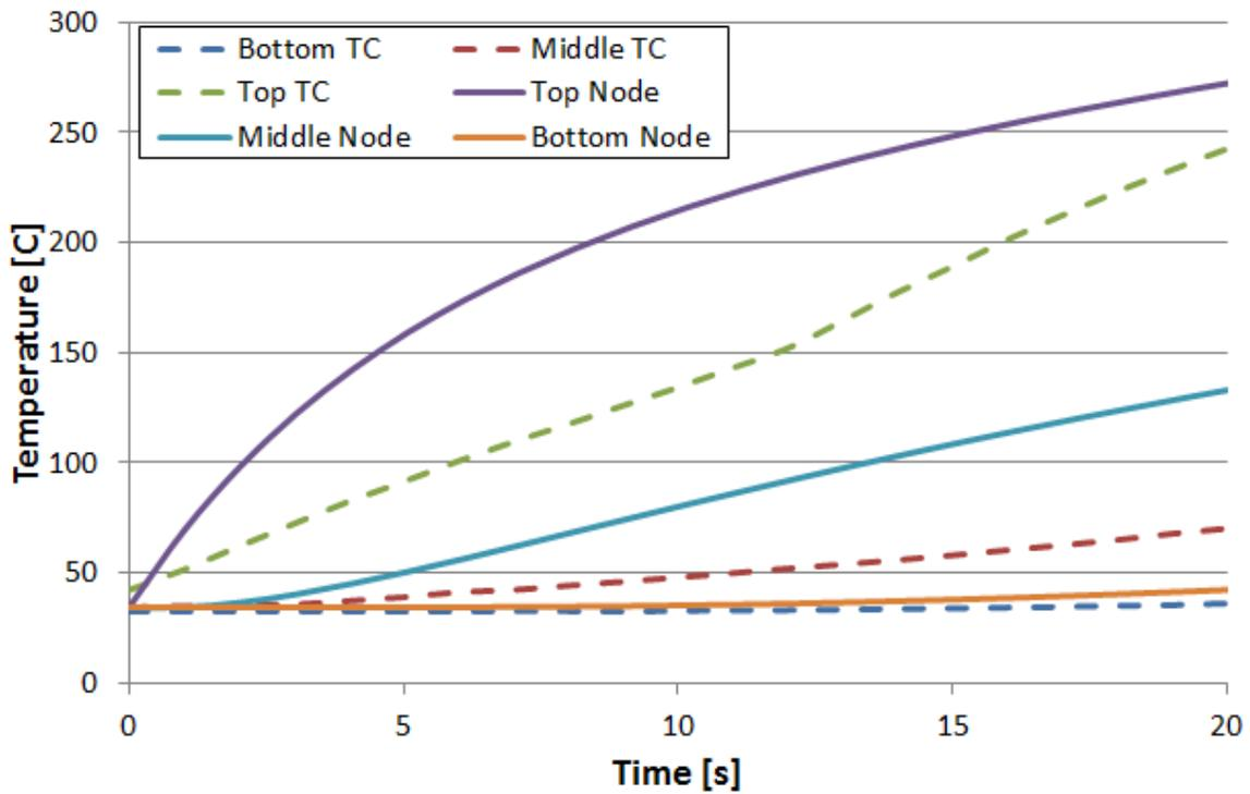
Figure 4.3.5: Boundary Condition 3 Temperature Distribution
