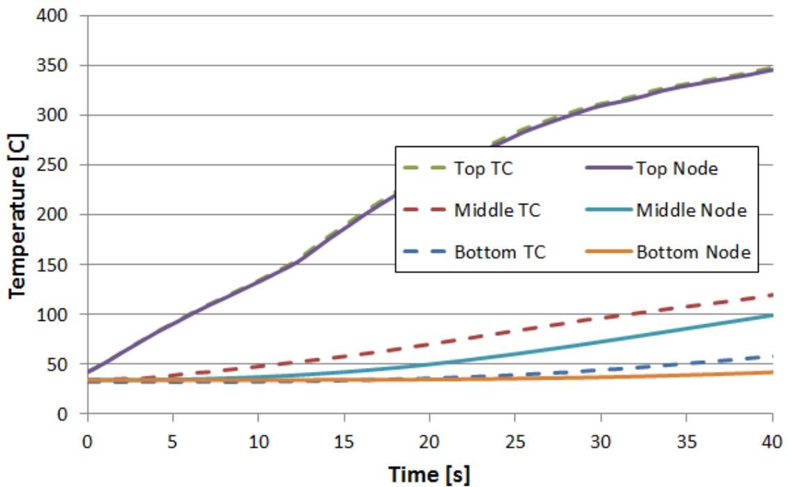
Figure 4.3.3: Boundary Condition 2 Temperature Distribution
