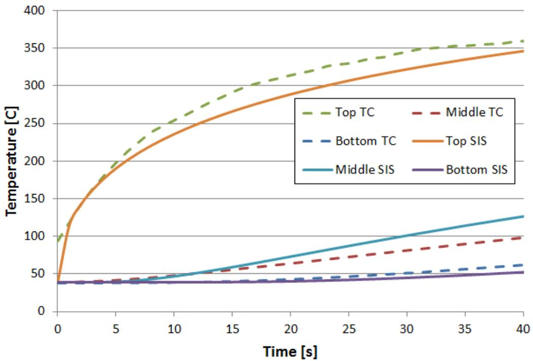
Figure 4.4.15: Boundary Condition 1 Temperature Distribution (SIS stands for Semi-Infinite Solid)
