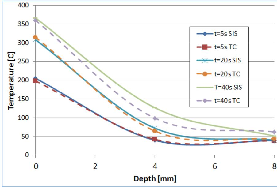
Figure 3.4.2: Temperature Profile for Kreysler System 1, BC-1 (SIS stands for Semi-Infinite Solids)
