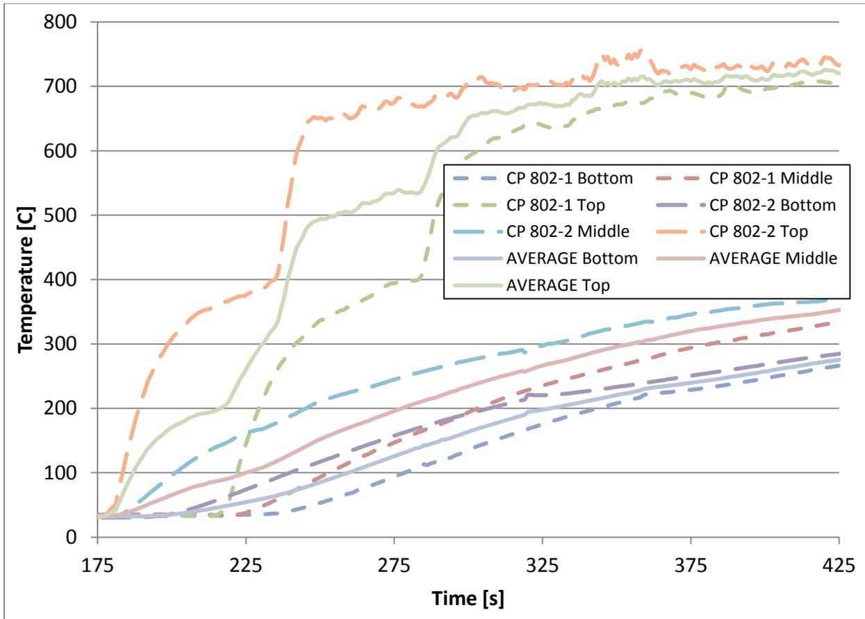
Creative Pultrusion      Skin 802      Test 1      50 kW/m<sup>2</sup>      10-25\_Sample4-1\_802\_50kW.txt
