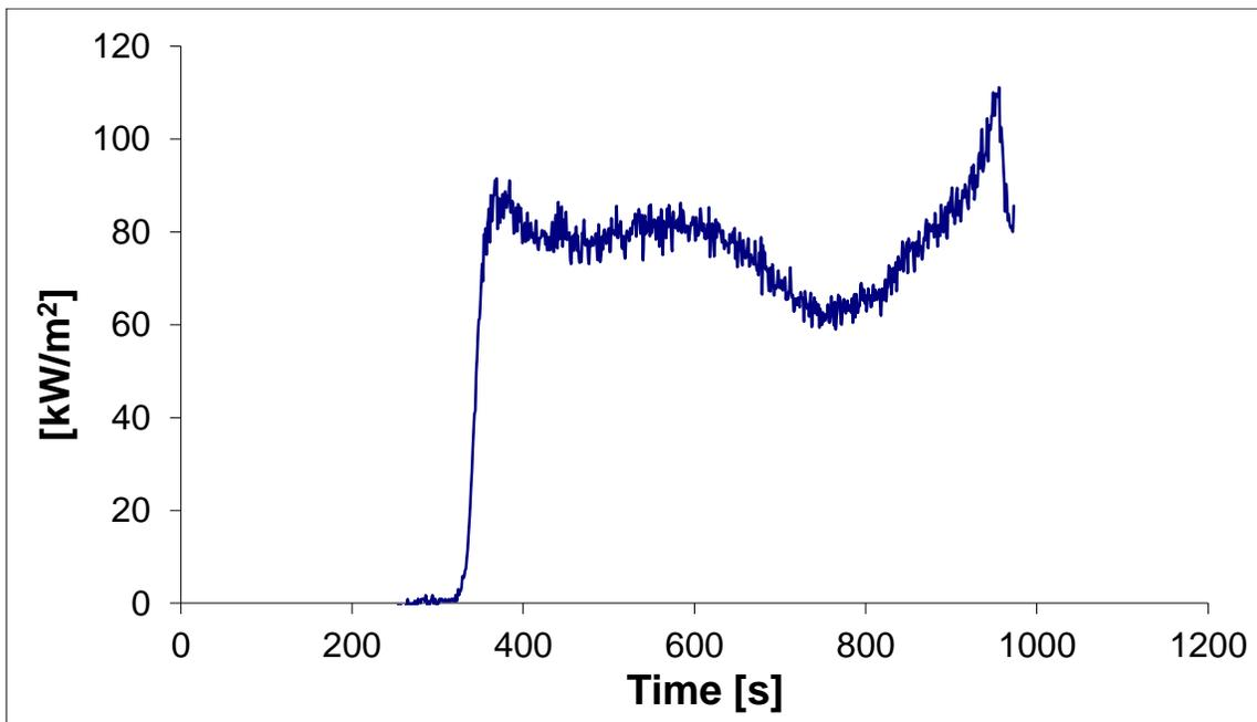
Figure 7: Heat Release Rate per Unit Area Kreysler 1, Test 2
