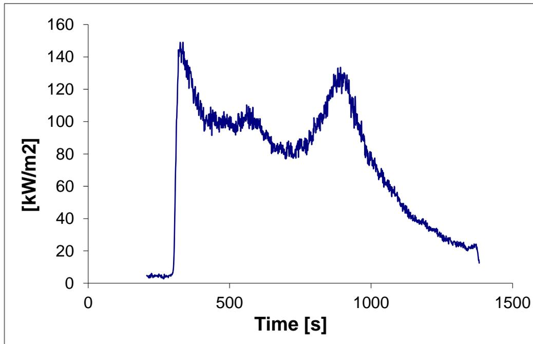
Figure 8: Heat Release Rate per Unit Area Kreysler 2, Test 1
