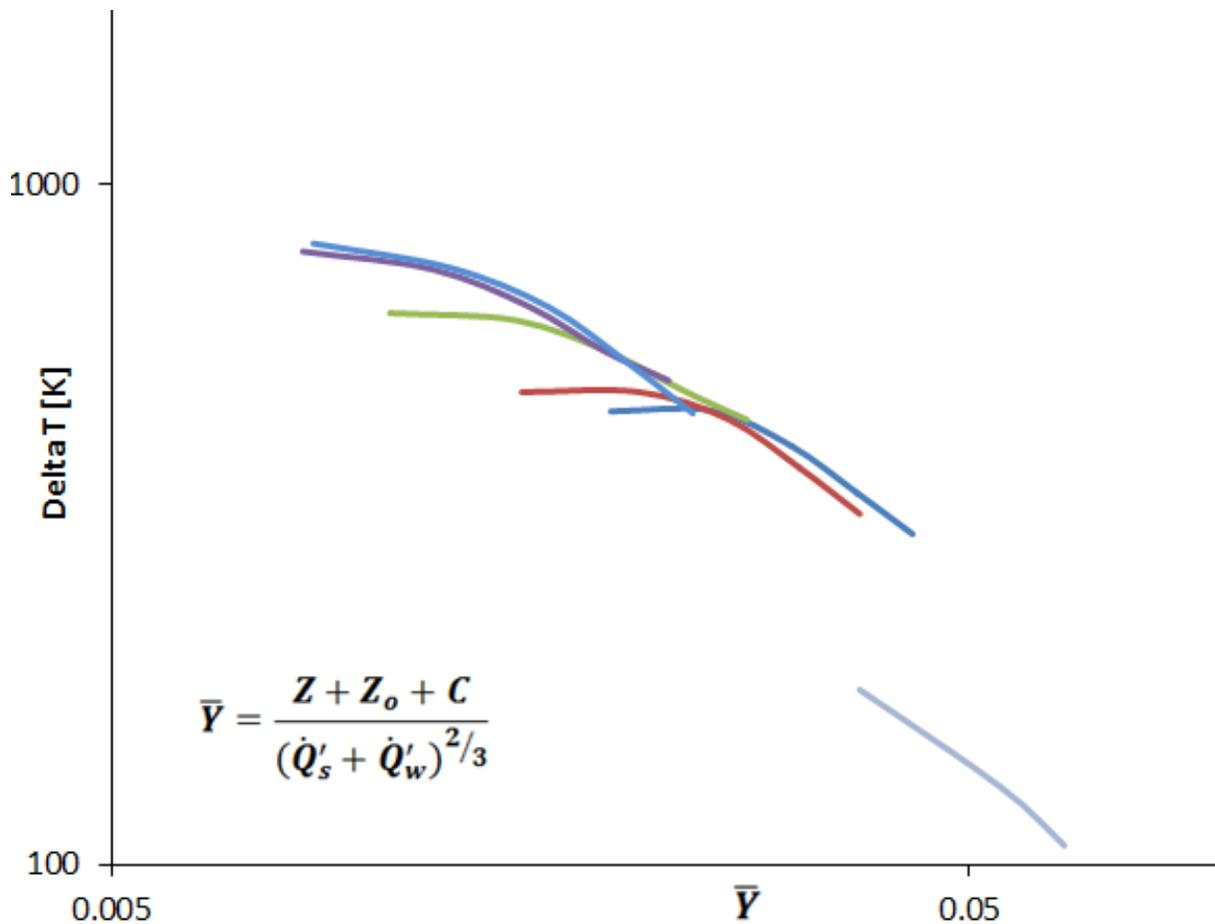
Figure 8: Graph of the test data for the 6 time steps after the heat release rates per unit length of the burning wall are estimated and added to the total heat release rate per unit length.
