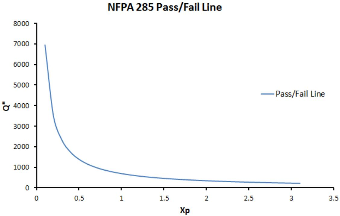
Figure 1: This graph demonstrates the prescriptive tool created to show the pass/fail curve for the NFPA 285 test. All combinations of  $Q''$  and  $x_p$  that fall below the curve indicate that the material would meet the acceptance criteria of NFPA 285, while pairs falling above the curve are not likely to comply.
