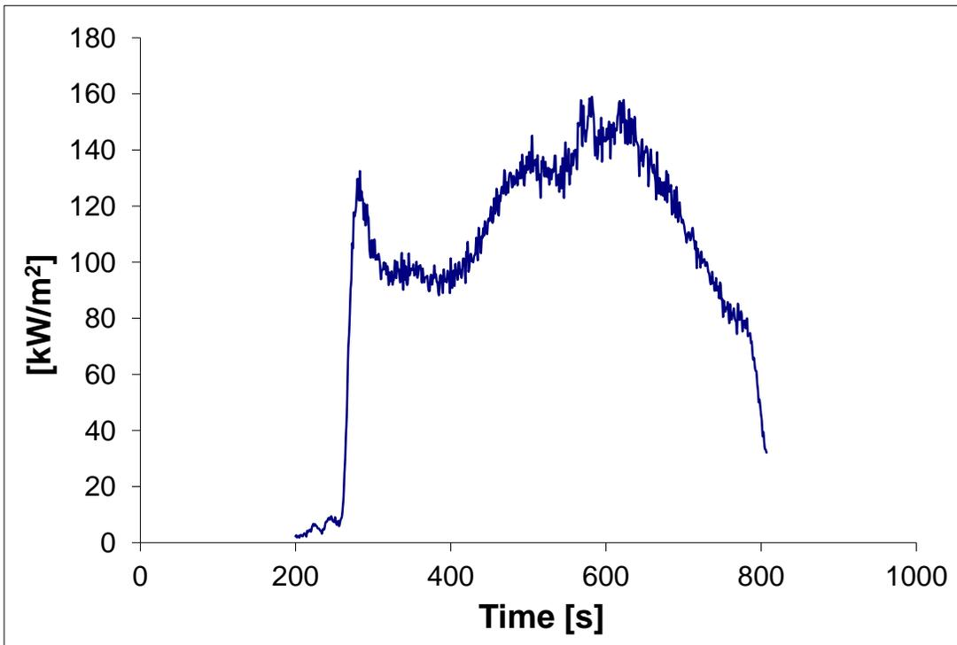
Figure 15: Heat Release Rate per Unit Area CP 286, Test 2
