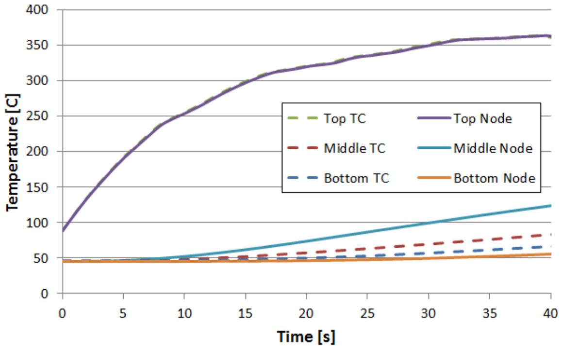
Figure 4.1.3: Boundary Condition 2 Temperature Distribution
