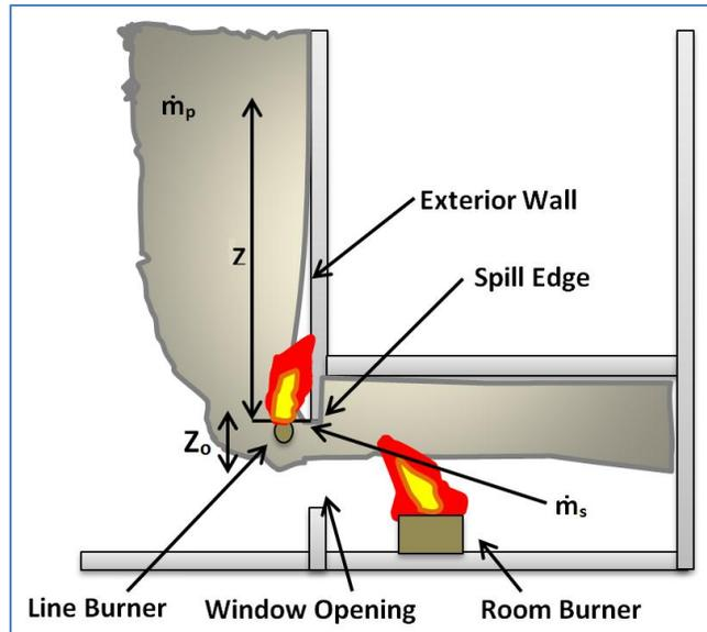
**Figure 2.1.2: Diagram of NFPA 285 test geometry**
