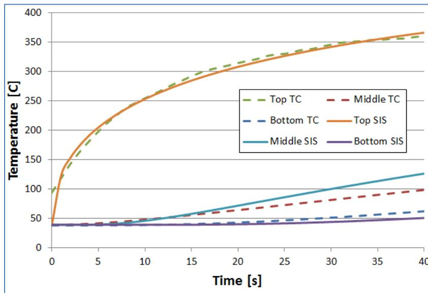
**Figure 3.4.1: Temperature Distribution for Kreysler System 1, BC-1 (SIS stands for Semi-Infinite Solid)**
