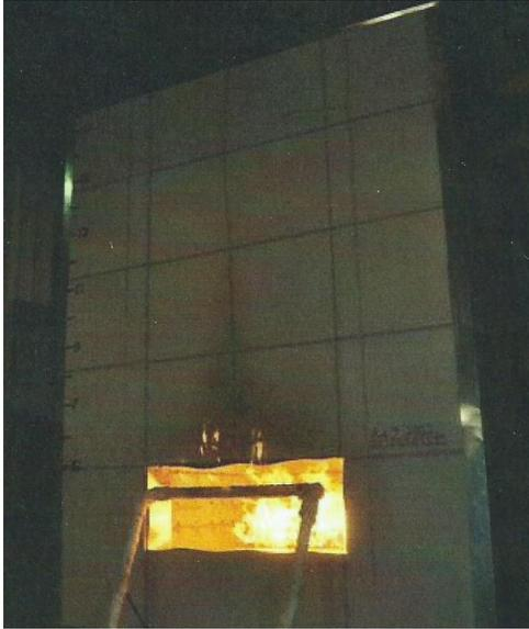
**Figure 4.2.1: Test photo taken at 7 min, 45 sec. No sustained flaming yet on the wall assembly.**
