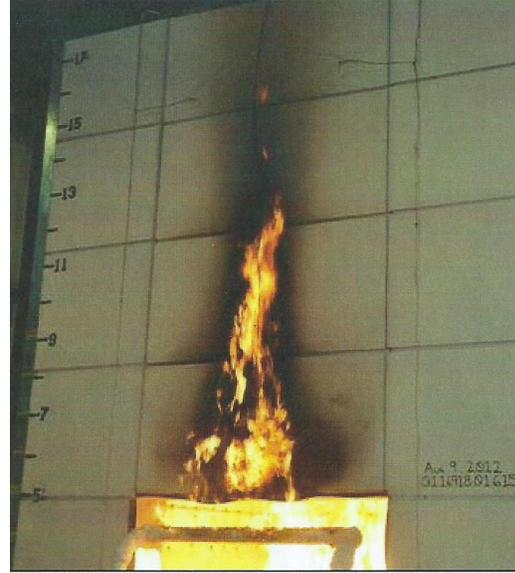
**Figure 4.2.2: Test photo taken at 21 min, 16 sec. Sustained flaming to approximately 11-ft mark.**
