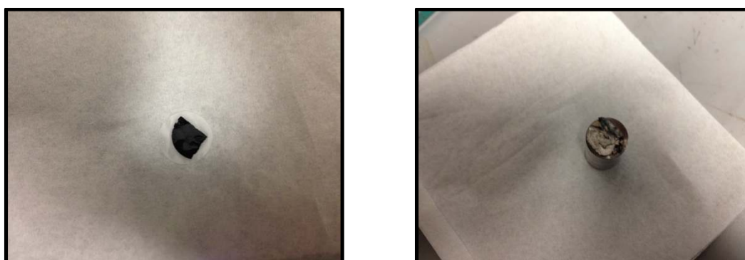
Figure 23: Left: LiCoO 2 cathode extracted after disassembly of cell, intact and reusable. Right: exhausted lithium metal anode preventing additional charging and discharging.
