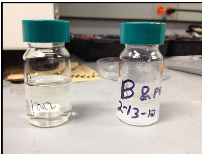
Figure 26: Comparison of PVP enhanced LLTO sol solution during the sol gel reaction sequence (left) and after the sol gel reaction sequence (right). Notice that the right vial has a thick precipitate and the left is clear.
