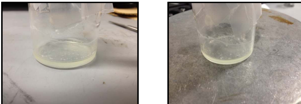
Figure 27: PVP enhanced LLTO sol solution thickened through partial evaporation. A thick slime and large particles are dissociated, indicating that partial evaporation is not stable enough to use for LLTO coating.
