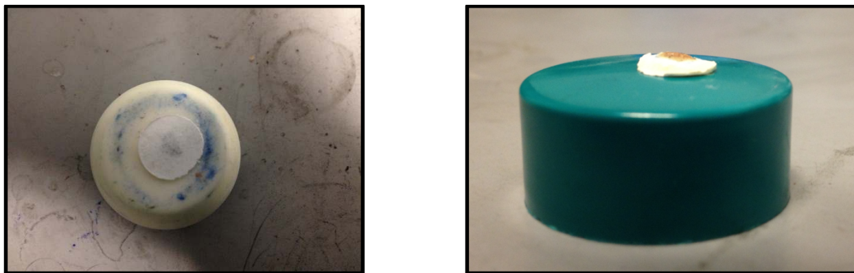
Figure 28: Flat, pre-heat treatment cold pressed LLTO powder on top of \text{LiCoO}_2 disk. Right: Deformed post-heat treatment LLTO disk with \text{LiCoO}_2 cathode removed.
