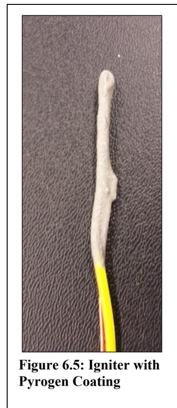
**Figure 6.5: Igniter with Pyrogen Coating**
