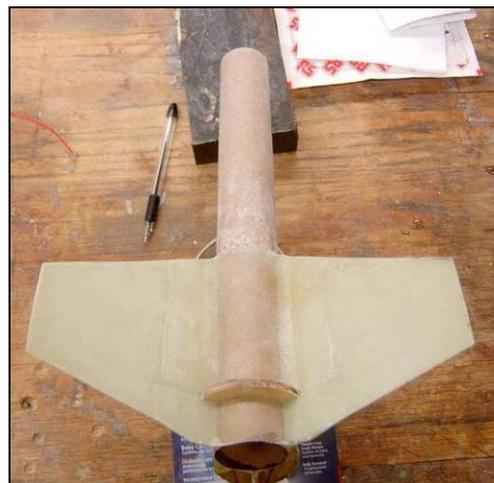
**Figure 3.19: Fiberglass Fillets to Motor Mount Tube**
