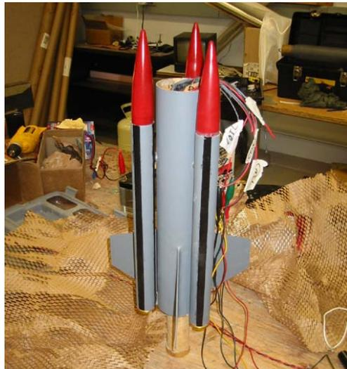
**Figure 4.50: Sub-Assemblies Link Together for Integrated Staging Systems Test**
