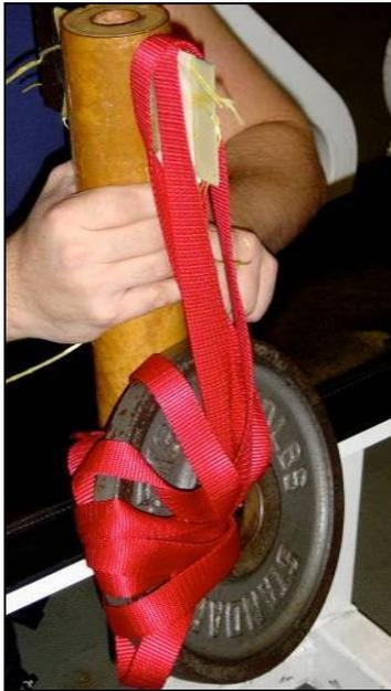
**Figure 3.8: Shear test for testing the merit of the fin attachment method**
