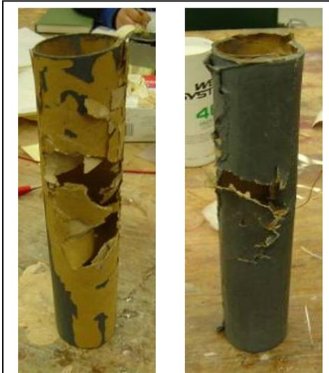
**Figure 3.26: Tubes A and B after the completion of the repeated normal force stress test**
