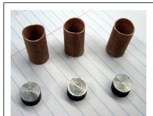
**Figure 4.34: Metal Retainers and Oversized Garolite Sheaths**
