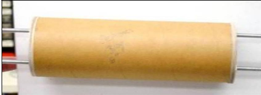
**Figure 3.11: Actual Electronics Bay (diameter of the coupler tube is 2.56 inches)**
