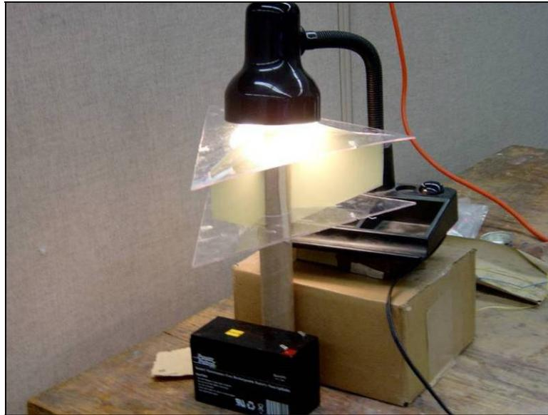
**Figure 3.18: The Heat Lamp Speeding Up the Curing Process**
