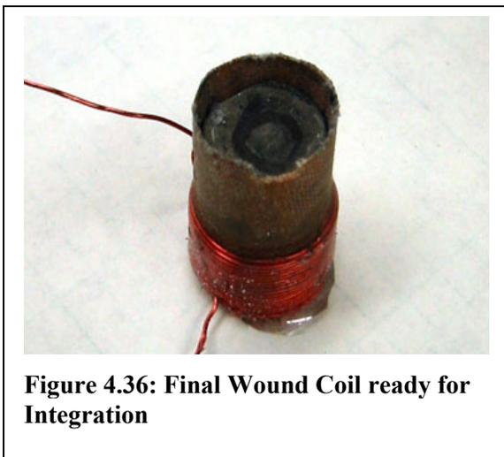
**Figure 4.36: Final Wound Coil ready for Integration**
