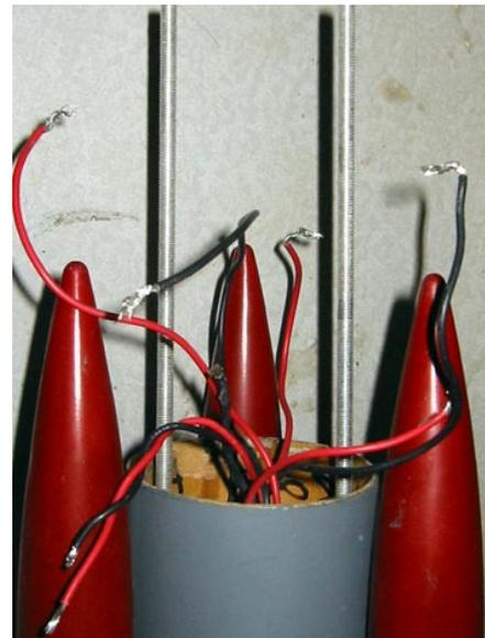
**Figure 4.46: Threaded Rod Installed at the Airframe Interface**
