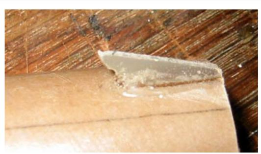
**Figure 4.28: Aft Hook attached to the prototype booster**
