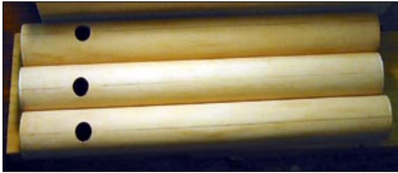
**Figure 4.35: Booster Airframes cut for Magnets**
