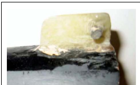
**Figure 4.33: Redesigned Aft Booster Hook**
