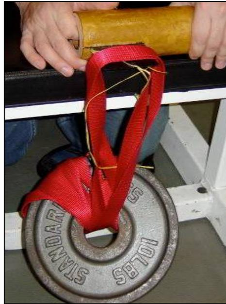
**Figure 3.9: Torque test for testing the structural merit of the fin material**
