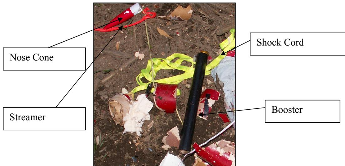
**Figure 5.20: Booster Recovery System (Post-Flight)**
