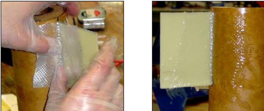
**Figure 3.7: The fiberglass cloth during and after application**
