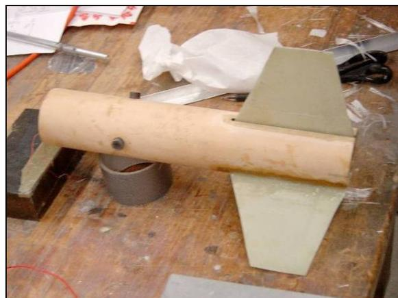
**Figure 3.21: Fiberglass Fillets from the Fins to the Airframe Tube**
