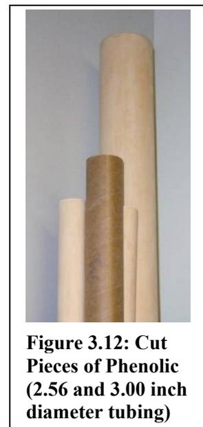
**Figure 3.12: Cut Pieces of Phenolic (2.56 and 3.00 inch diameter tubing)**
