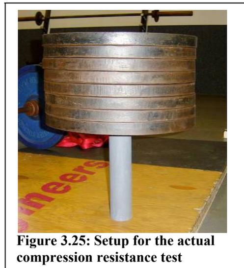
The repeated normal force stress test, despite the use of a simple testing method, allowed the structural integrity of the body tubes to be easily observed. Applying repeated instantaneous forces brought both tubes to failure. Tube A failed at a much faster rate and endured a higher level of
