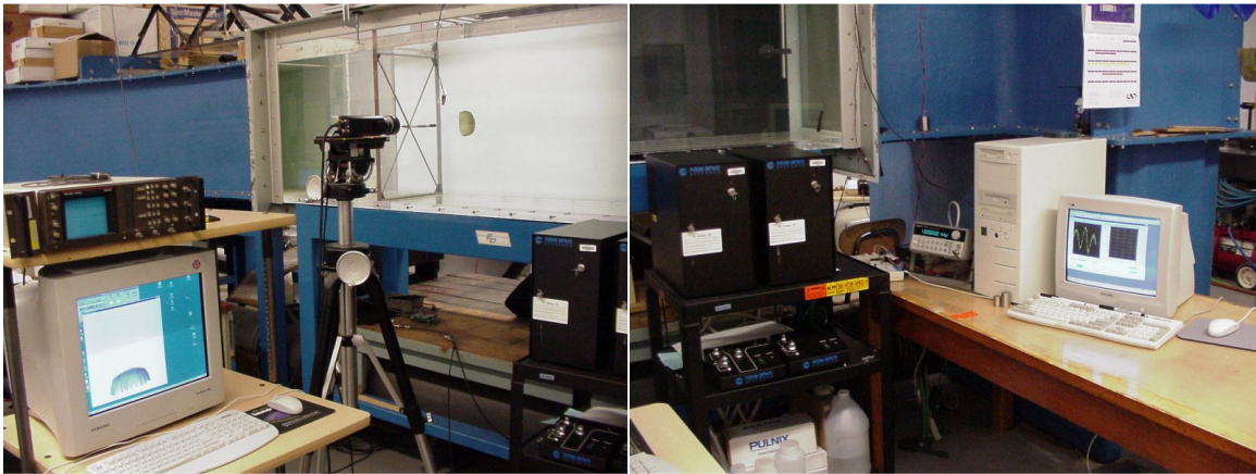
a) b) Figure 2.2. Photographs of experimental setup, a) imaging computer, camera, and parachute model in water tunnel; b) data acquisition computer and lasers used in DPIV system.
