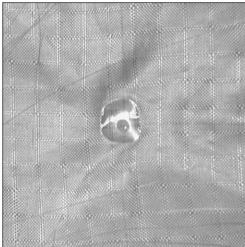
Figure 2.7. Close-up image of hard grommet at apex of canopy.
