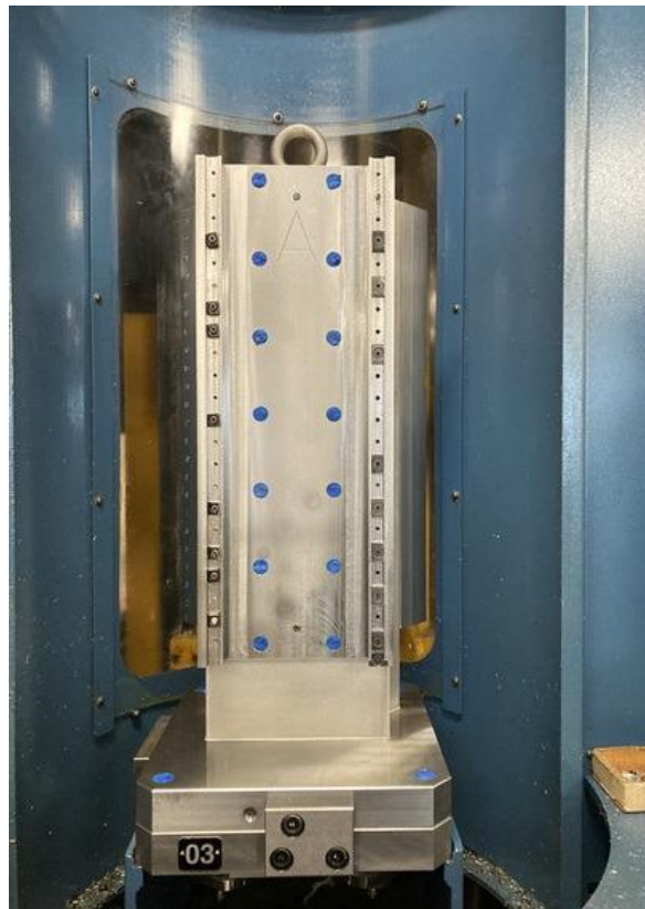
Figure 2.3 – Tombstone #3 in Sjogren’s Matsuura H-Plus 300, viewed from Face A.
