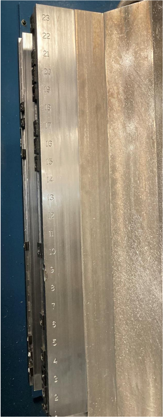
Figure B-1 – Stop numbers 1 through 23 on the Matsuura H-Plus 300's Tombstone #3 Face C.
