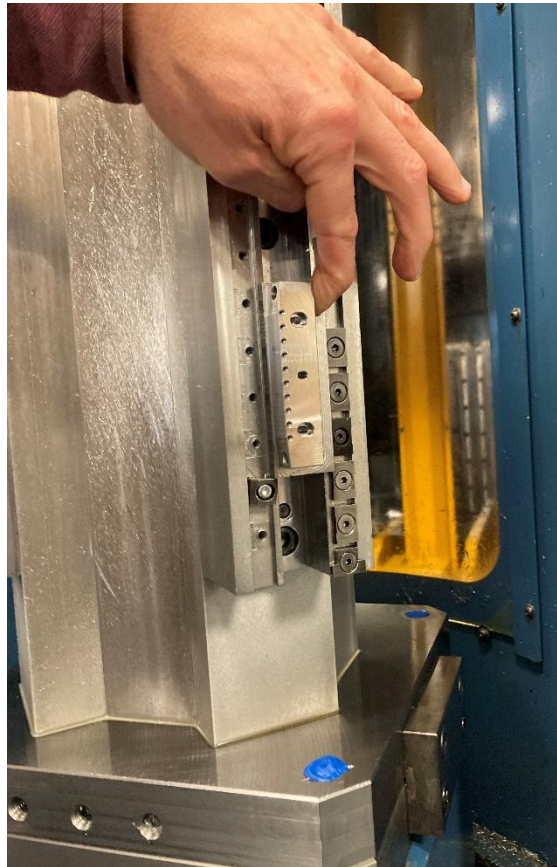
Figure 2.4 – Cut material being placed into the third stop on Face C of Tombstone #3.
