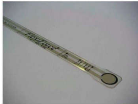
Figure 4-35 Piezo resistive Force Sensor [49]
