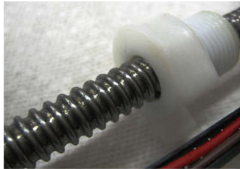
Figure 4-15 Schematic of a screw drive mechanism.
