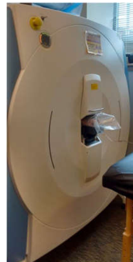
Figure 7-5 (a) shows the specimen loaded in the device (b) shows the device loaded into the CT scanner
