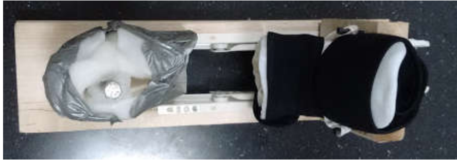
Figure 4-18 Updated tension design including the gripping mechanisms
