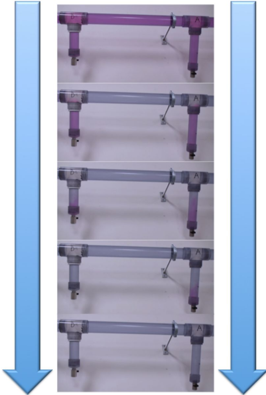
Figure 9: Visible Mixing Over Time in Dead-Leg “A” Compared to Dead-Leg “B”
