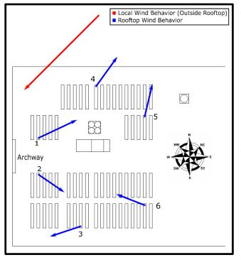
unpredictable. To the left is a diagram showing the wind speeds and directions measured on the farm. Wind speed is indicated by the arrow lengths. From this, we learned that the wind barriers would have to protect crops from all angles. Interviews with other urban rooftop farmers revealed that another farm in Toronto has experienced wind damage to their tomato plants in the past. This showed that the wind problem at Higher Ground Farm is not unique.
