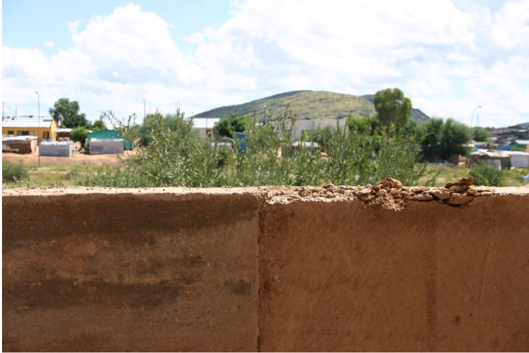
Figure 7: Compacted soil wall samples at the Habitat Research and Development Centre. Left half shows compacted soil with four percent concrete. Right half shows compacted soil with no cement.
