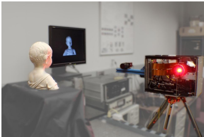
Fig. 4.7. Realization of system setup on a tripod viewing a sculpture for measurement.
