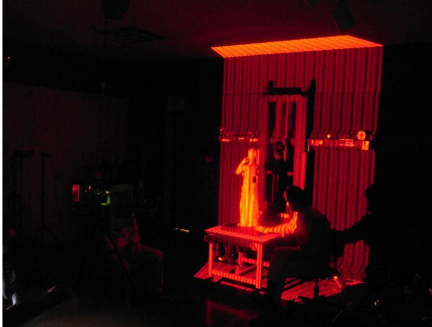
Fig. 7.17. Projection system FOV at approximately 2 meters form the Orant sculpture.
